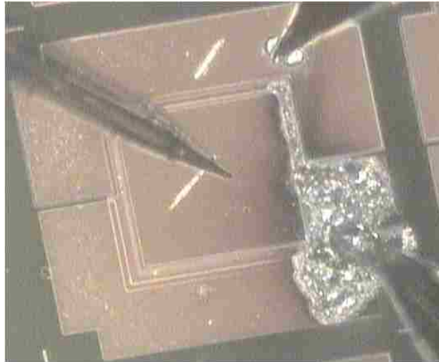
Figure 7.14: A top view probe-station microscope image of a completed 3-terminal \text{SiO}_2 passivated gated diode (square mesa size of 400\mu\text{m} and no aperture) under overload condition, with all three probes attached.
