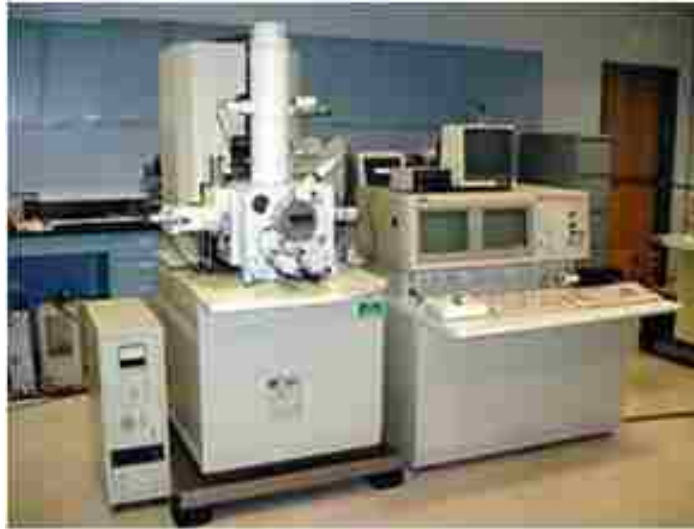
Figure 2.9: Photograph of JSM 6400 field emission scanning electron microscope (FESEM) instrument.
