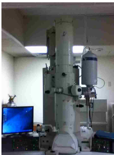
Figure 2.8: Photograph of JEOL 2010 200kV high resolution transmission electron microscope (HRTEM) instrument.
