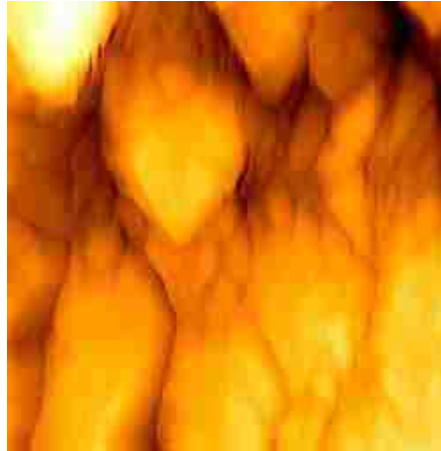
Figure 4.2: AFM image on 1 \mu\text{m} \times 1 \mu\text{m} area of InAs substrate etched with \text{H}_2\text{O}_2:\text{HCl}:\text{H}_2\text{O} (1:1:4) solution.
