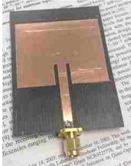
Figure 3.16: Fabricated 2.2GHz patch antenna.
