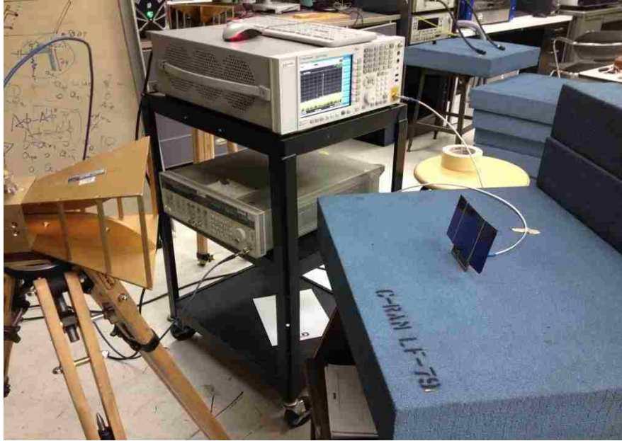
Figure 5.9: Photograph of the test performed with solar cell covering the front of the antenna underneath the PIFA design.
