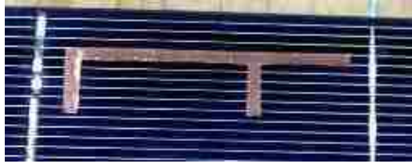
Figure 5.4: PIFA design cut from copper tape for solar cell integration.
