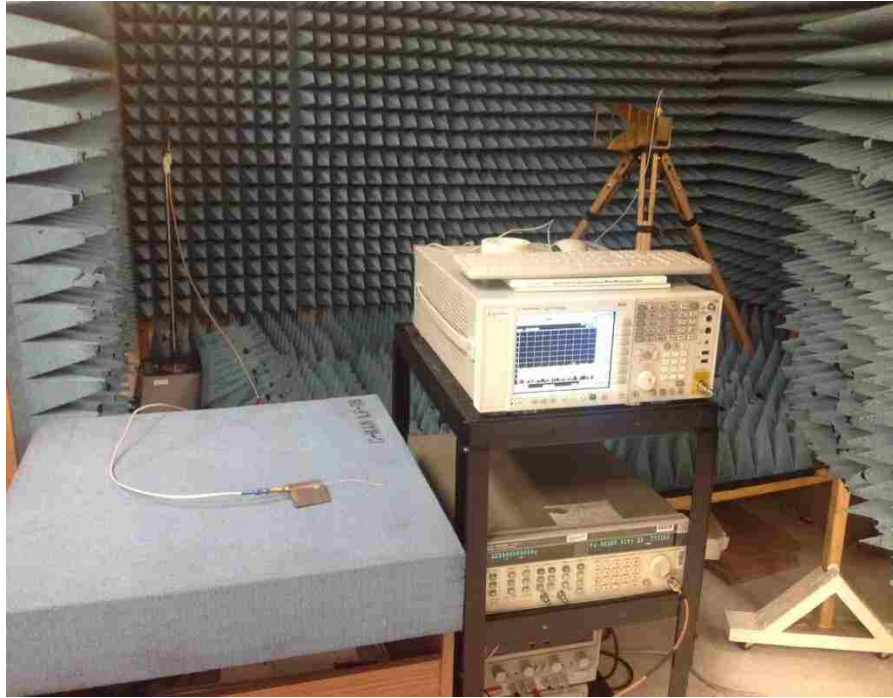
Figure 3.27: Photograph of the setup for the antenna measurements using a 2.22 GHz patch antenna.
