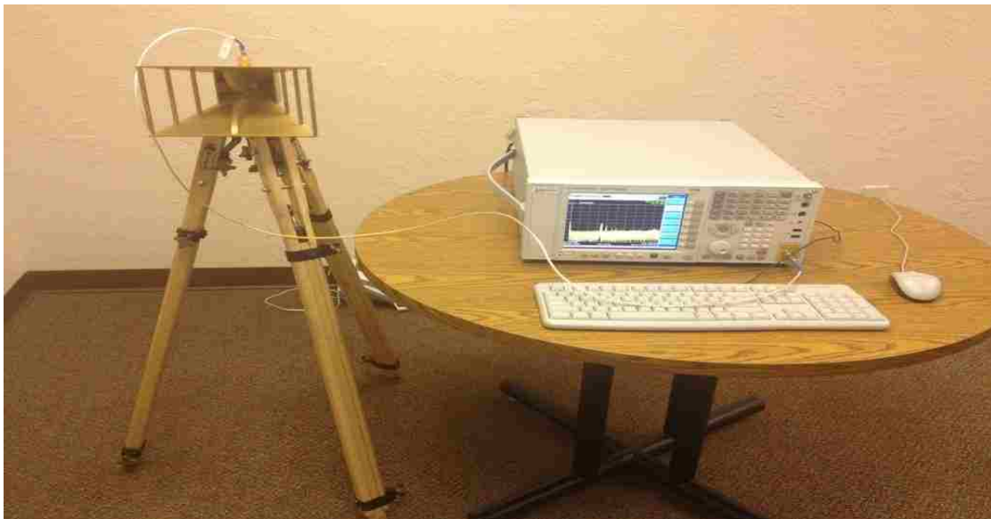
Figure 3.2: Setup for spectrum analyzer measurements.
