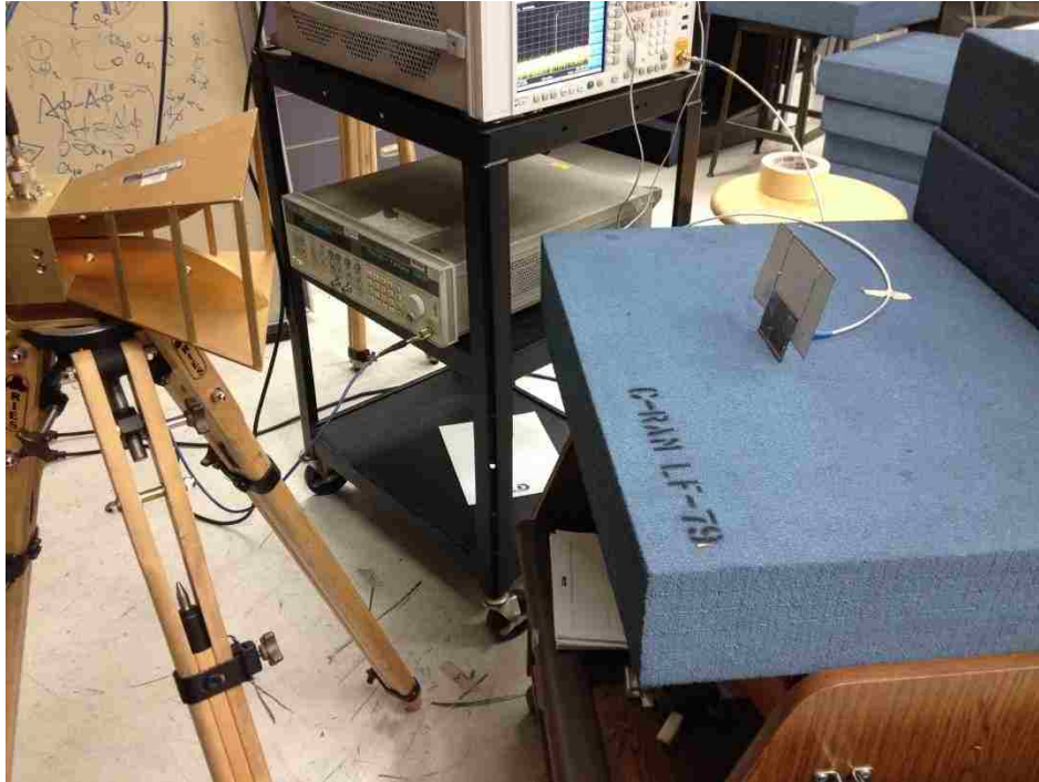
Figure 5.8: Photograph of the test performed with solar cell covering the ground plane of the antenna
