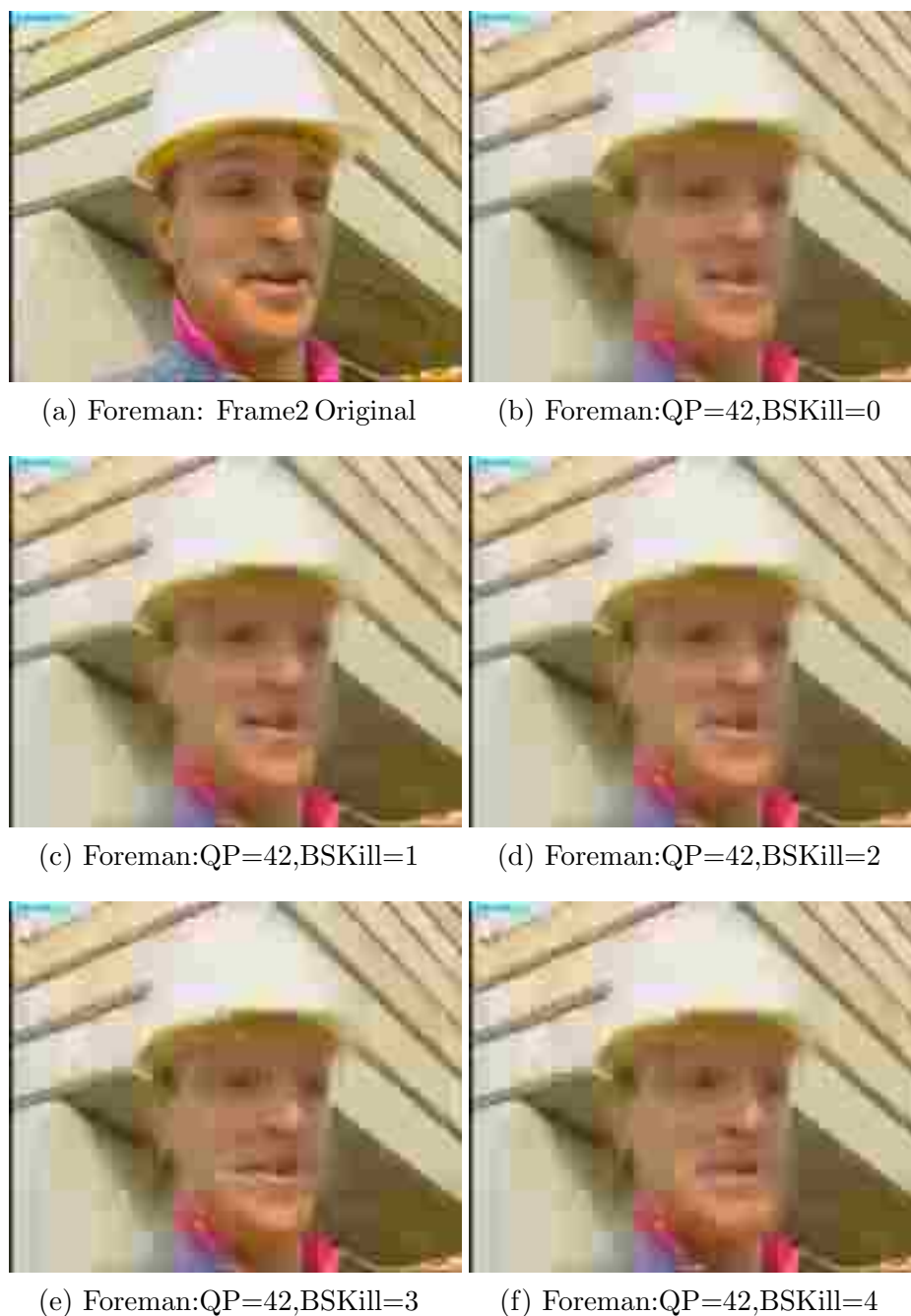
Figure 4.4: Deblocking filter results for foreman video frame 2 where DBF works as expected. In this example, we are using H.264/AVC JM 18.2 with QP = 42 . We demonstrate the results for: (a) original image, (b) BSKill = 0 gives SSIM=0.8182 , (c) BSKill = 1 gives SSIM=0.8155 , (d) BSKill = 2 gives SSIM=0.8145 , (e) BSKill = 3 gives SSIM=0.8005 , and (f) BSKill = 4 gives SSIM=0.7882 .
