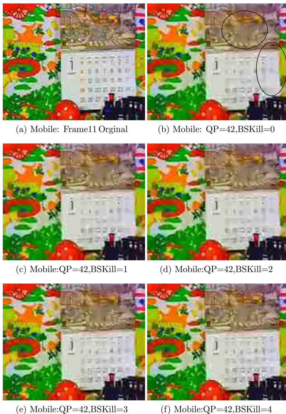
Figure 4.5: Deblocking filter results for mobile video frame 11 where DBF can perform worse than expected. In this example, we are using H.264/AVC JM 18.2 with QP = 42 . We demonstrate the results for: (a) original image, (b) BSKill = 0 gives SSIM=0.7203 , (c) BSKill = 1 gives SSIM=0.7199 , (d) BSKill = 2 gives SSIM=0.7194 , (e) BSKill = 3 gives SSIM=0.7358 , and (f) BSKill = 4 gives SSIM=0.7365 . To see the effects of over-filtering, compare the two ellipsoidal regions shown in (b) with the original image in (a), and the rest of the sub-figures.
