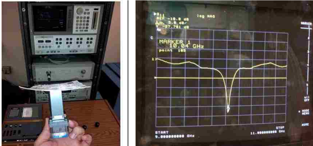
Figure 50: Fabrication and measurement of the 10GHz antenna
