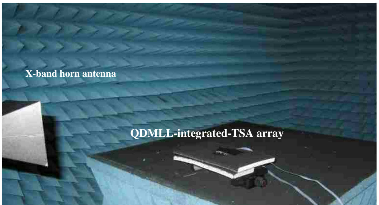
Figure 4.30 Photo-image of the measurement setup
