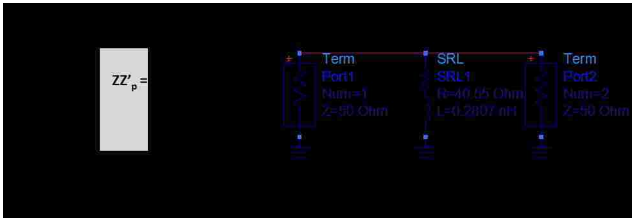
Figure 3.8 (a) Simplified \pi -network model (b) Equivalent lumped circuit
