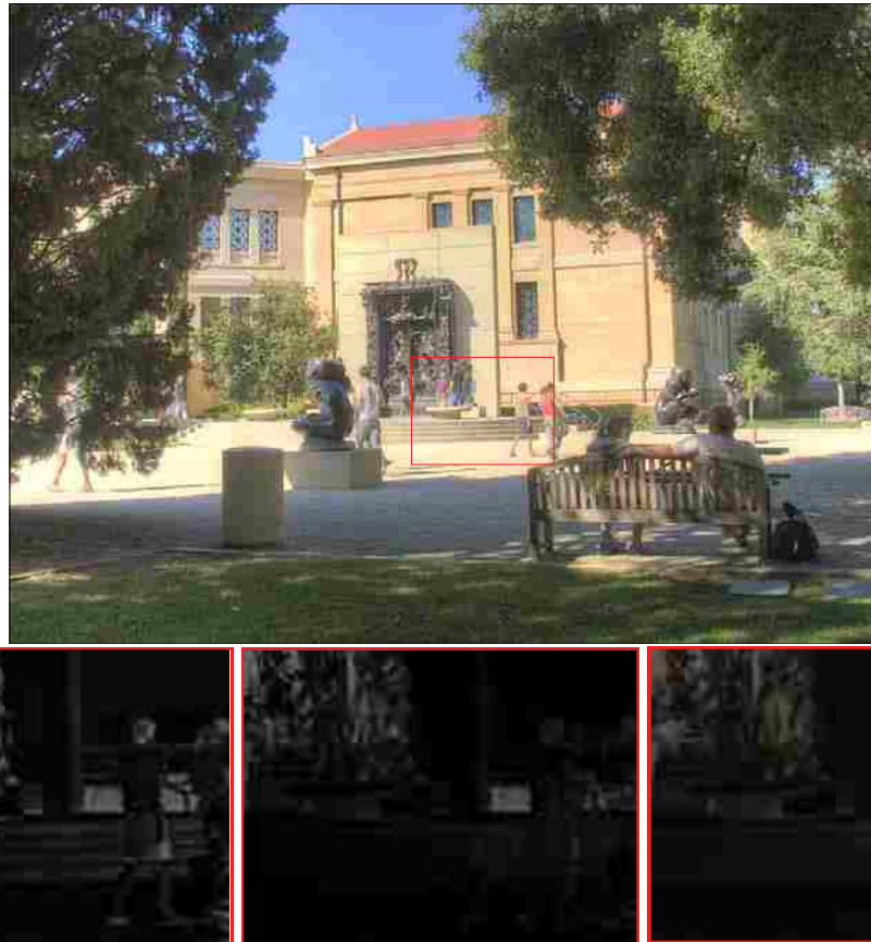
Figure 4.12: This scene (from Gallo et al. [2009]) has moving people that are different in every frame. We show the results of the deghosting methods of Gallo et al. (left) and Pece and Kautz [2010] (middle) using images provided by the authors. The former has visible block artifacts because of the way they detect motion in a per-block basis, and the latter leaves much of the ghosting. Our method (top and right) can remarkably reconstruct most of the moving people, but it has artifacts as well. These appear as “washed out” regions where our algorithm only had information from one LDR image because the people in the reference disappeared.
