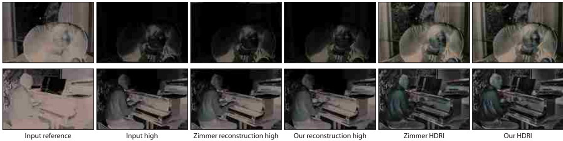
Figure 4.13: Here we compare the reconstruction and HDRI results of our method with Zimmer et al. [1] method. We gave the images to the authors and they ran their code on them. Zimmer et al. method is not able to reconstruct the moving objects (e.g. the man and reflection of him on the piano) which appears as ghosting in the final HDR image. Our method, however, can produce high quality results.
