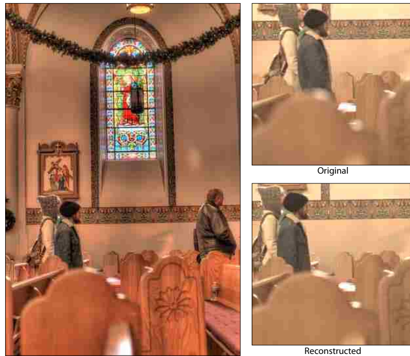
Figure 4.10: This figure shows how our algorithm can sharpen an image to match the the depth of field of the reference. For this scene (our HDR result shown on the left), we captured 10 stops of bracketed exposure by changing both the aperture as well as shutter time. This was the only way to take this picture since the camera was hand-held. On the right we show one of the original input frames, as well as our reconstruction. We see that the out-of-focus region on the bench has been made sharper to match the reference.
