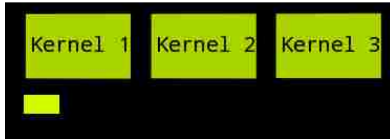
Figure 3.1: CUDA's Default Stream Behavior
