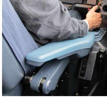
Figure 3.2: Right seat armrest showing the sidestick on an A-330 aircraft [1].
