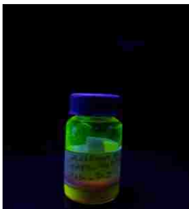
Figure 2.7: Synthesized CdSe/ZnS DS QDs emitting around 570 nm (greenish-yellow), under the UV lamp.
