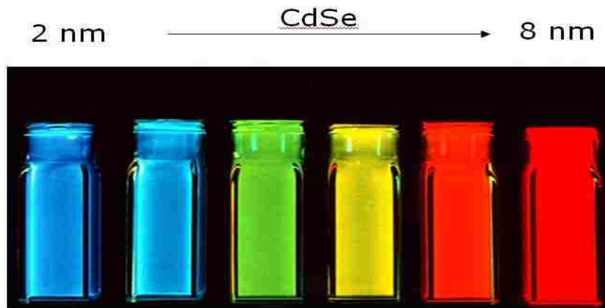
Figure 1.2: Colloidal quantum dots irradiated with a UV light. Different sized quantum dots emit different color light due to quantum confinement (Bawendi, 2014).
