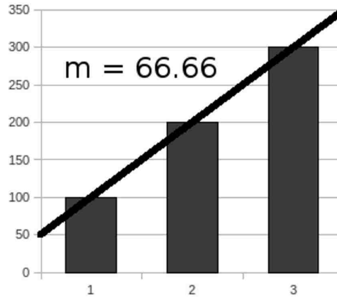
Figure 5.2: Example of the technique used to determine radiation threats with the slope of linear regression with a histogram.
