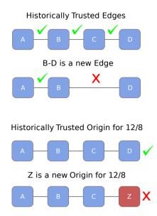
Figure 3.3: Examples of anomalies. First, AS path (A,B,C,D) has been seen in a recent route. Therefore edges  $A \rightarrow B$ ,  $B \rightarrow C$ , and  $C \rightarrow D$  are in the normal database. Next, a route update with AS path (A,B,D) is received, which has an anomalous edge  $B \rightarrow D$ . In the next example, AS D is in the normal database as the origin of prefix 12.0.0.0/8. The new route update has Z for the origin AS, which is anomalous.
