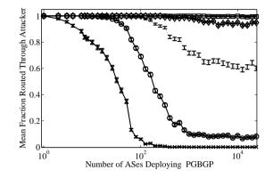
Figure 4.2: Worst case propagation of a new sub-prefix over time. The bottom line shows the immediate suppression of the new sub-prefix by PGBGP. The X-axis shows the number of ASes that have deployed PGBGP (in decreasing order of degree) and the Y-axis represents the fraction of ASes that select routes through to the sub-prefix. Each successive line above the bottom line represents the propagation of the sub-prefix one day later.
