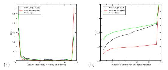
Figure 4.3: Length of stay in the RIB for anomalies. Anomalies that exist within the RIB at twenty-four hours are added to the normal database and considered trusted. Panel a shows the probability mass function while panel b shows the cumulative distribution function. Only the largest feed was used for this experiment.
