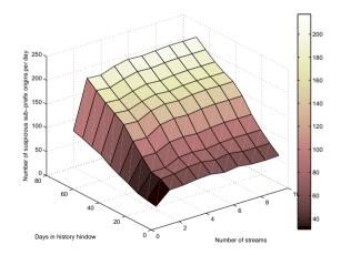
Figure 4.5: The number of sub-prefix hijack anomalies, or alerts, that PGBGP observed during the 4 month time period. The initial h days were used to initialize the normal database. The figure represents a parameter sweep of the number of BGP streams and the duration of the history window h.
