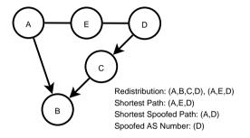
Figure 2.2: Examples of invalid paths. Autonomous System A modifies its AS path when exporting routes to gain access to D's traffic. The paths listed in the legend are those that A could send to its neighbors for each type of invalid path attack. Arrows point to customers from providers, and undirected edges represent peer-peer relationships.
