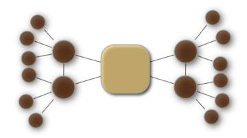
Figure 6.7: Betweenness centrality. The middle node does not have the greatest degree, but it is along the greatest number of shortest paths.
