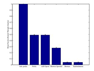
Figure 4.1: Effectiveness of each synthetic attack against a network of ASes without any security protection using the standard export rules. The x-axis describes the form of attack simulated while the y-axis represents the fraction of ASes that routed through the adversarial AS after 500 simulated attacks. Error bars represent standard error of the mean.
