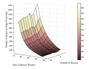
Figure 4.6: The number of edge anomalies, or alerts, that PGBGP observed during the 4 month time period. The initial h days were used to initialize the normal database. The figure represents a parameter sweep of the number of BGP streams and the duration of the history period h.
