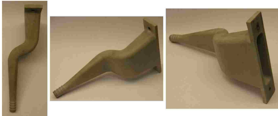
Figure 2.8: Three photographs of the suction manifold fabricated using stereolithography and used in the experiment. The end with the rectangular opening and flanges was attached to the bottom of the shock tube directly below the nozzle location. The suction was supplied through a flexible hose that was attached to the circular section with the hose barb connection.
