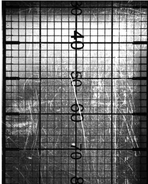
Figure 3.6: Calibration grid for the DYN camera. Served as the control image for the orthogonal mapping of IC camera images.
