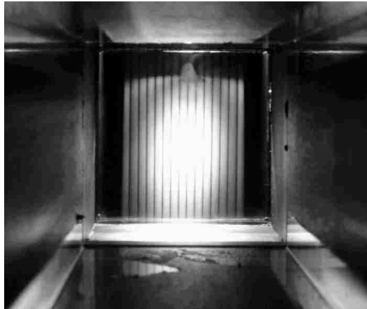
Figure 2.3: Photograph of the axis view of the shock tube (looking through the window at the end of the end section) showing the varicose curtain initial conditions flowing from top to bottom. Visualization was accomplished with fog droplets for flow seeding in the \text{SF}_6 and a flashlight for illumination.
