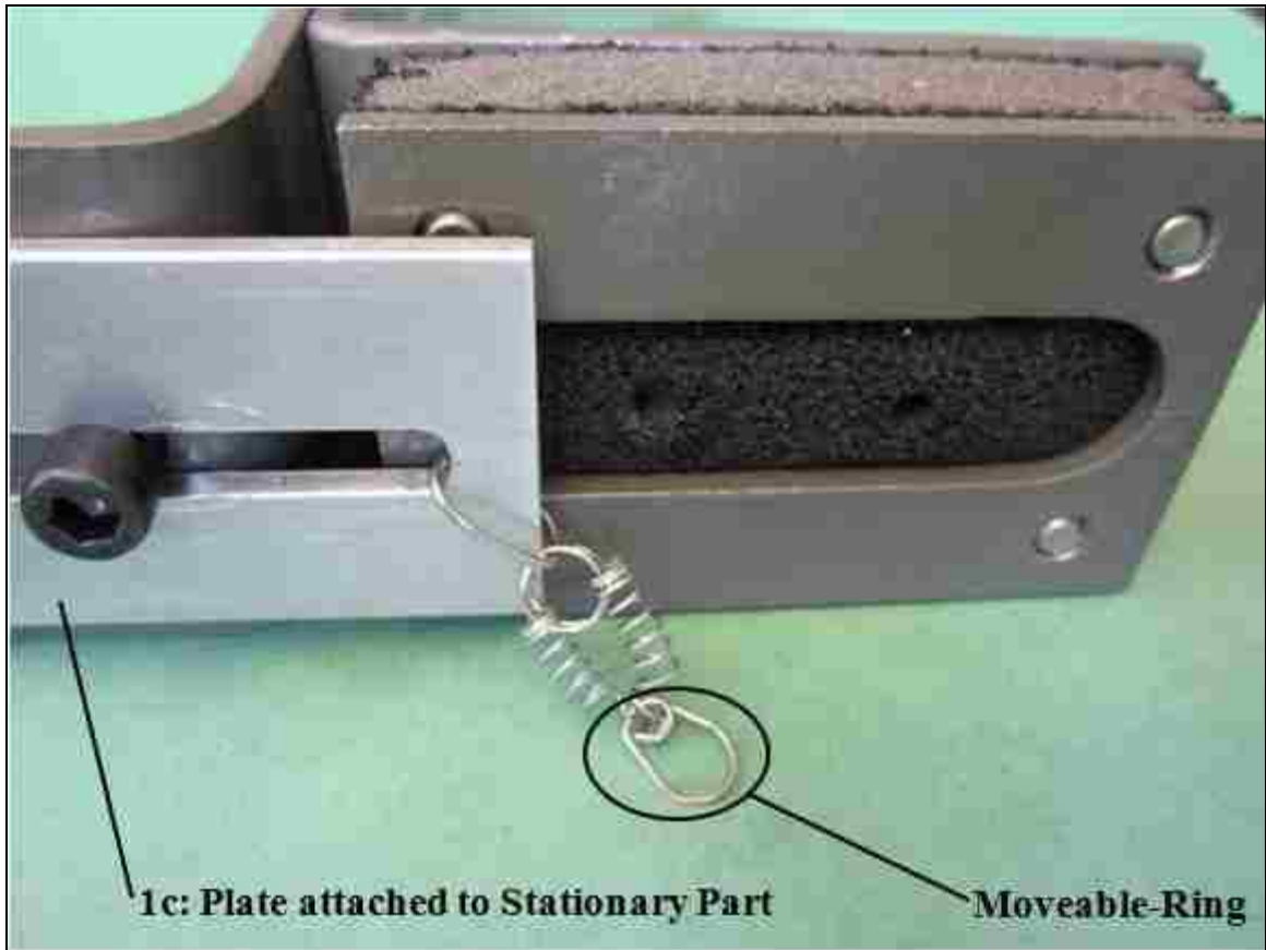
Figure 25: Moveable-Ring utilized as the moveable point of Suture Attachment.
