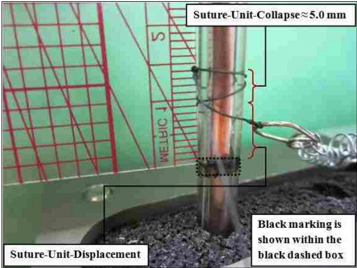
Figure 34: The RS Suturing-Technique reaching a Suture-Unit-Displacement of 9.0 mm.
