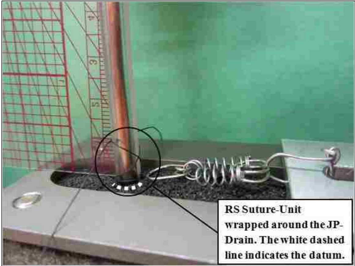
Figure 28: RS Suturing-Technique with 1.0 cm initial separation between the LB and the second Knot-Unit used in the research setting.
