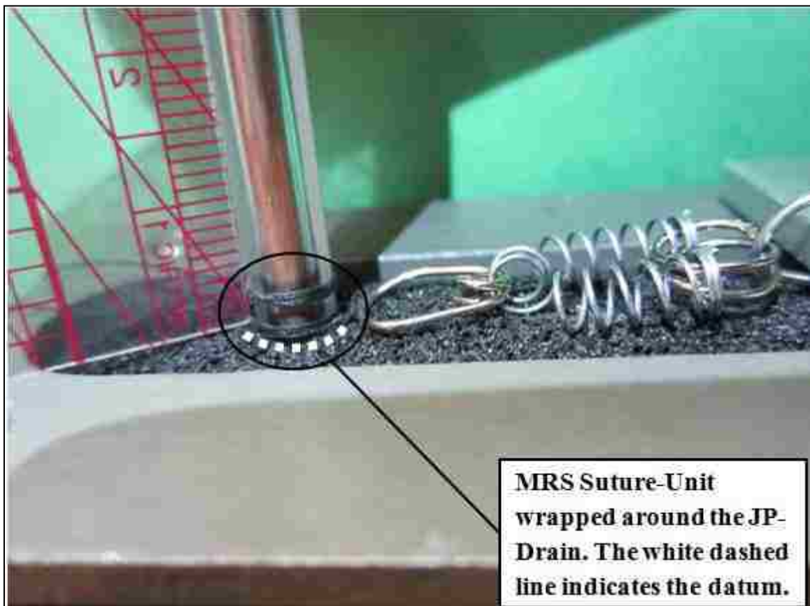
Figure 31: MRS Suturing-Technique with 2.5 mm initial separation between the LB and the UB used in the research setting.
