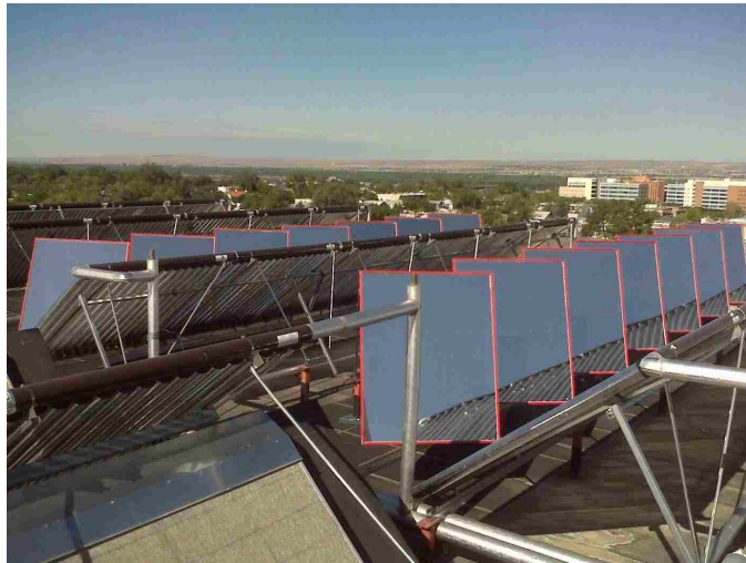
Figure 2.11: Mirrors in the background are set at \alpha = 30^\circ and \beta = 42^\circ and mirrors in the foreground are set to \alpha = 20^\circ and \beta = 42^\circ
