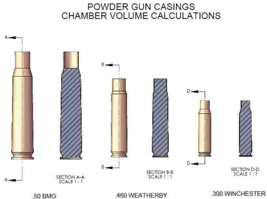
Figure 22. 0.50 Cal Powder Gun Casings
