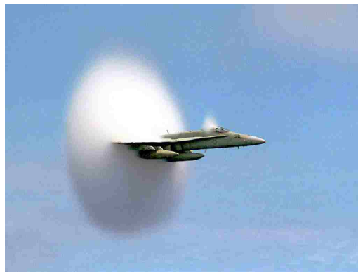
Figure 1.1: A stationary shock wave forms on the wing of an aircraft, causing large flow deceleration and subsequent vapor condensation [3].
