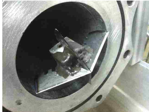
Figure 3.3: Image of the puncture head used to rupture diaphragms between the driver and driven sections of the shock tube.
