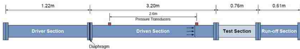
Figure 3.1: Schematic of UNM Shock Tube.
