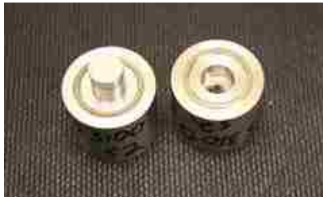
Figure 2-12: Shear napkin ring test geometry.
