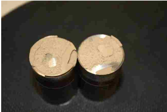
Figure 2-13: Butt tension test geometry.
