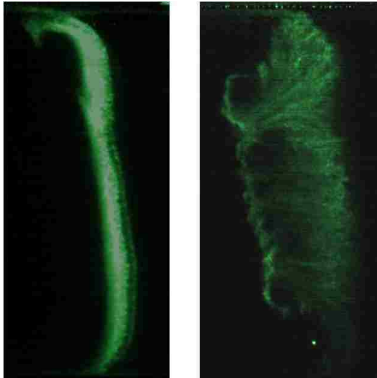
Figure 6.5: Side view of the glycol droplet-seeded air column (left) and the glycol droplet-seeded SF 6 column (right) at late times, roughly 650 \mu s after shock passage. The image extends the full height of the shock tube, i.e. 75 mm. [2]
