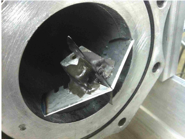
Figure 3.2: The four-pointed star puncturing head, mounted in the driver section.
