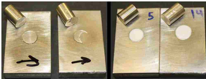
Figure 13 - Failure at H = 0.374'' (unfilled at left, 40vol% alumina filled at right)
