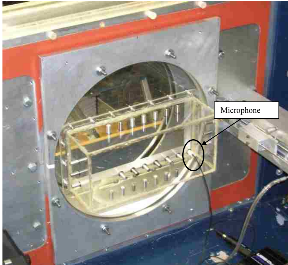
Figure 7: Cavity 1 mounted to the TBLG with microphone at the downstream location on the floor of the cavity.
