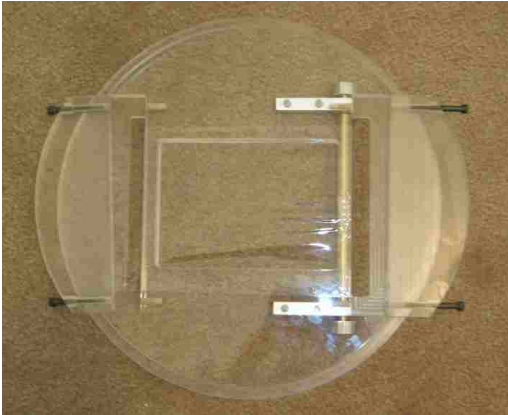
Figure 8: Film clamping assembly showing three pieces that comprise the window, the film stretched across the rectangular hole, and the tension rod (on the right).
