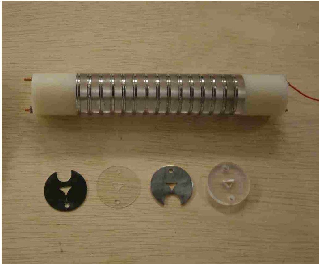
Figure 18: Photo of an assembled electrode stack with stainless steel electrodes and polycarbonate insulators.
