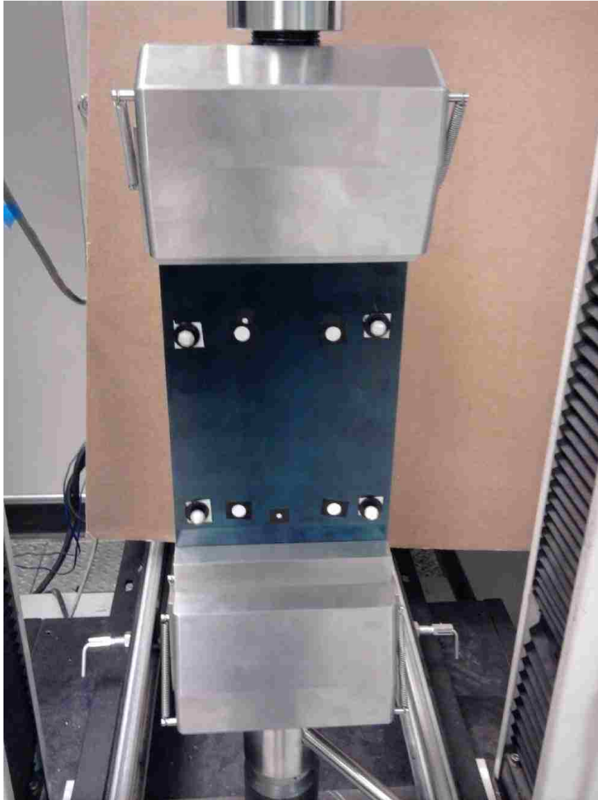
Figure 55. Sample for front-plane movement tests. Includes two kinds of retro-reflective targets for increased confidence in the results; spheres and circles.
