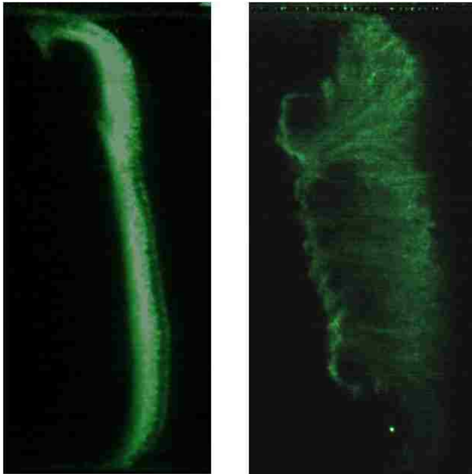
Figure 7.3: Experimental images in the vertical plane of the air-fog (left) and SF 6 -fog (right) instabilities at M=1.67, 19.05 cm downstream.
