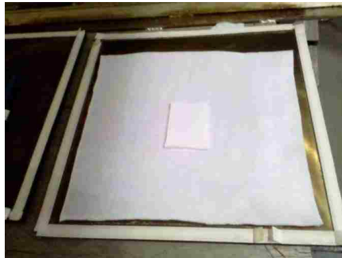
Figure 3-13: N-10 Placed on top of caul plate
