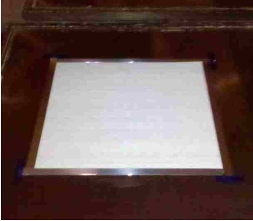
Figure 3-11: S2 fiber glass panel surrounded with shims on a caul plate
