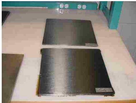
Figure 3-16: Cured carbon fiber plates with resin flash on the sides
