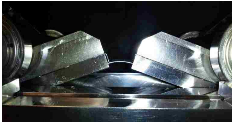
Figure 3-3: Carbon fiber laminate specimen in pure bending
