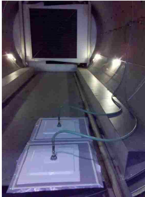
Figure 3-15: Panels ready for cure in autoclave
