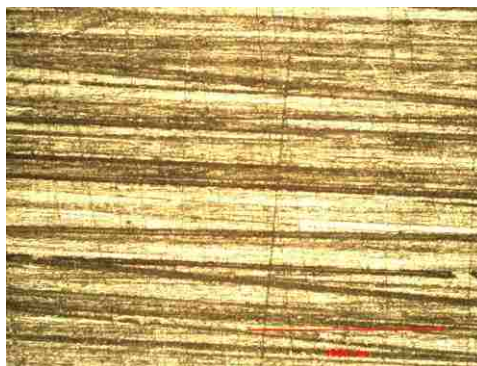
Figure 3-7: Surface of a cured new style IM7/8552 plate x5 magnification
