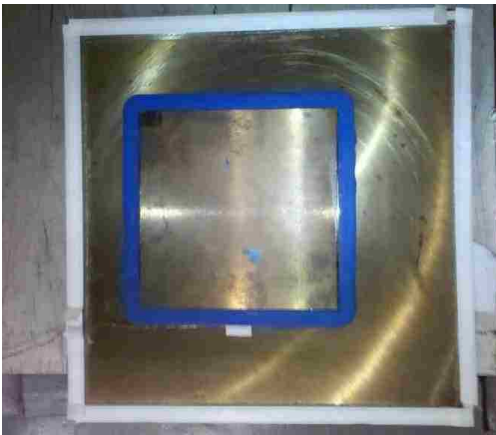
Figure 3-12: Rubber dam around a caul plate with a thermocouple
