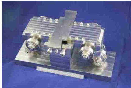
Figure 3-19: Carts in the alignment fixture with adjustable parallels setting the gage length
