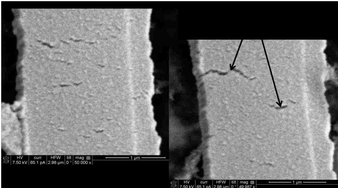
Figure 5.9: Intergranular fatigue cracks along the length of the 250nm thick test film subjected to fatigue loading.
