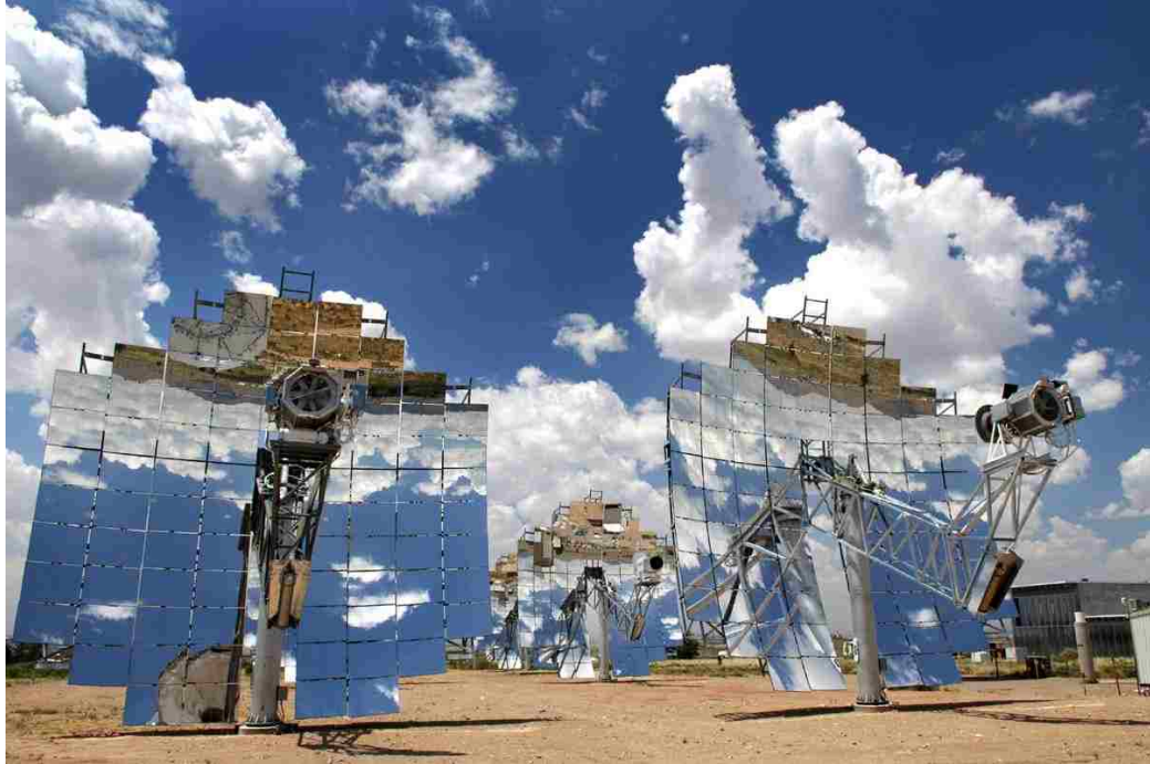
Figure 2. Stirling Energy Systems (SES) CSP dish technology. Credit: Sandia National Laboratories/Randy Montoya. Copyright: 2008 Used by permission. Location: Albuquerque, NM (US Department of Energy 2012).
