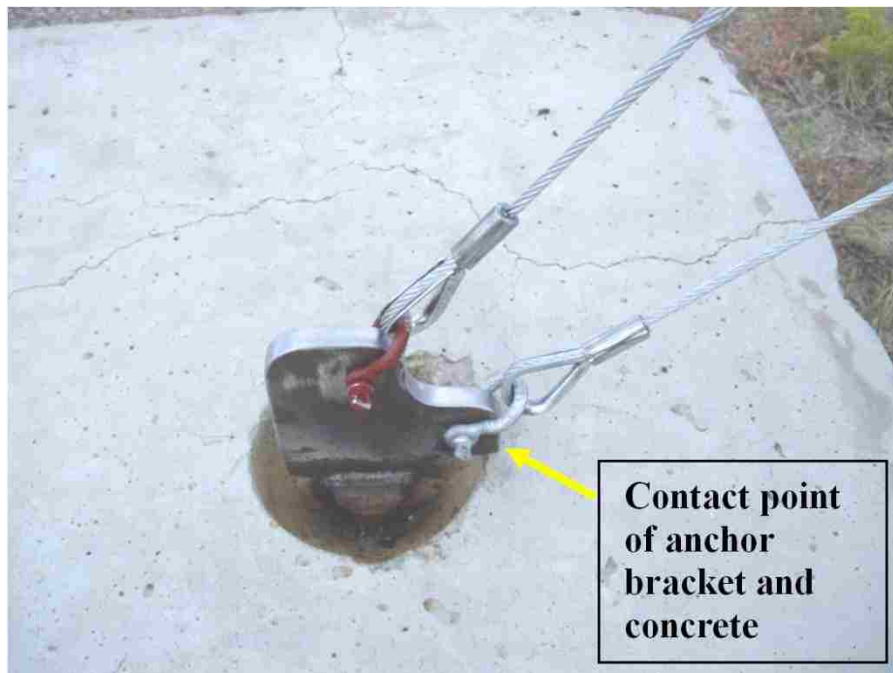
Figure 12: Anchor bracket welded to lifting pin. Contact point between bracket and concrete is made to mitigate bending stress on the lifting pin.
