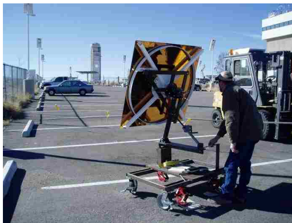
Figure 26: Single facet rig. Operator is holding the turnbuckle used as an azimuth drive.
