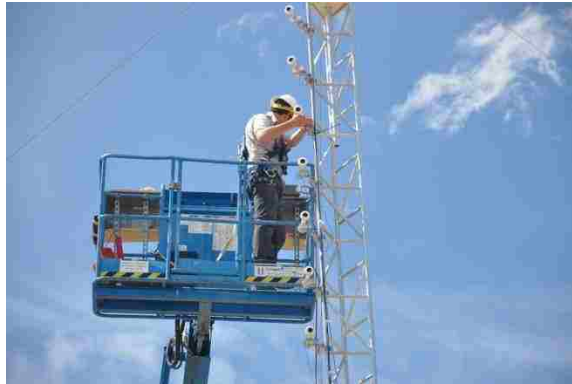
Figure 21: Author aims sensor at a light source. (Sment, Ho, et al., Flux Characterization for Long-Distance Heliostats 2012). At sufficient distance the heliostat beam is not dangerous.
