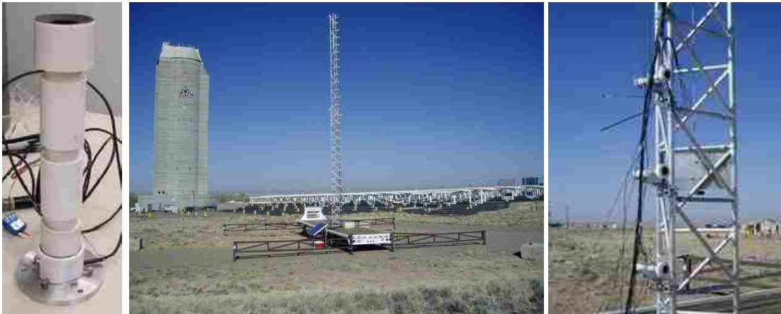
Figure 15: Left: Collimated LI-COR pyranometer. Middle: Photo of trailer-mounted mobile heliostat target with NSTTF central receiver tower in background. Right: close-up of collimated pyranometers mounted on aluminum tower.
