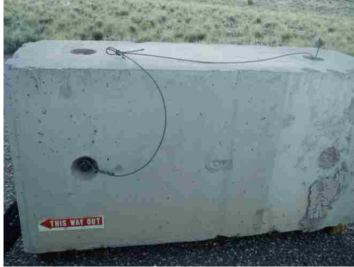
Figure 10: 2400 kg concrete anchors 61x91x1.5 cm (2x5x3 ft) were available at no cost. Analysis was performed to show functional equivalence to ground anchors and safety of handling.
