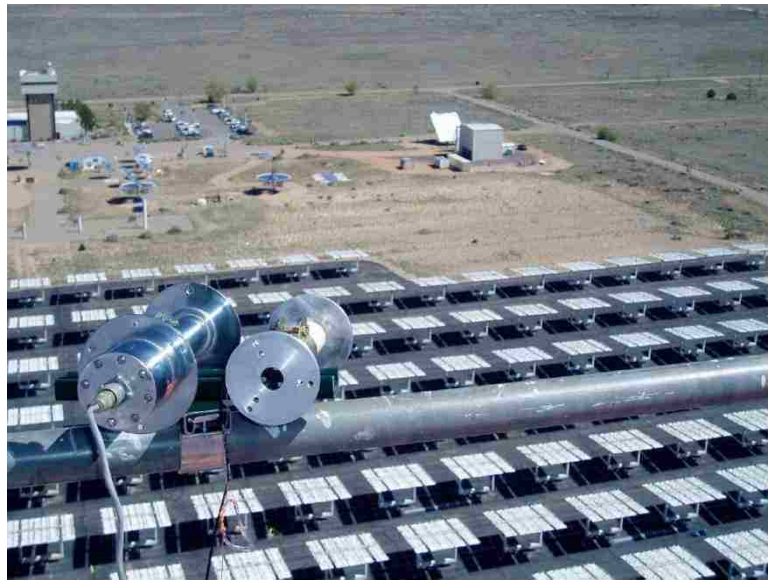
Figure 16: Eppley NIP (left) and Collimated LI-COR LI-200 (right) are aimed at a heliostat to test for response time. (Fisher 2010)
