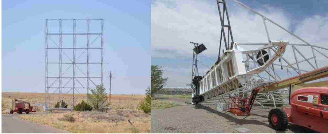
Figure 7: (Left) First prototype of long distance target erected on trailer. (Right) Wind-blown target has flipped trailer causing significant risk to safety and capital loss.
