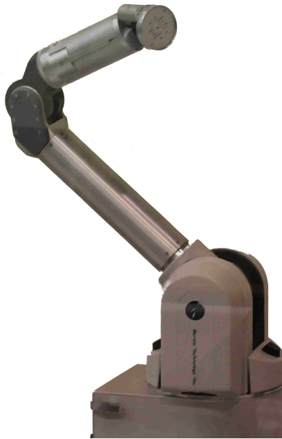
Figure 3.2: Whole Arm Manipulator by Barrett Technologies
