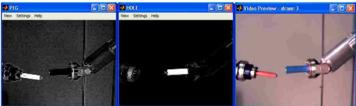
Figure 6-2. Binary images produced by the vision system after color filtering with the calculated pixel coordinate location of the tip of each part marked by an “X”. The figure on the right shows the actual color image that was input into the system by the camera.
