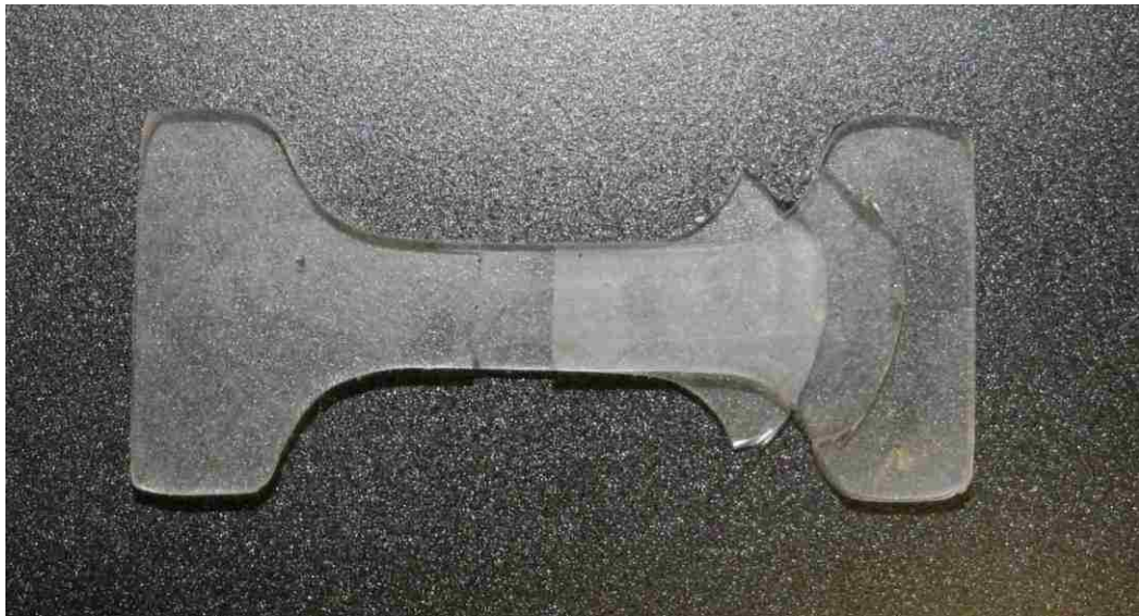
Figure 18. Example of de-lamination that occurred during tension testing.
