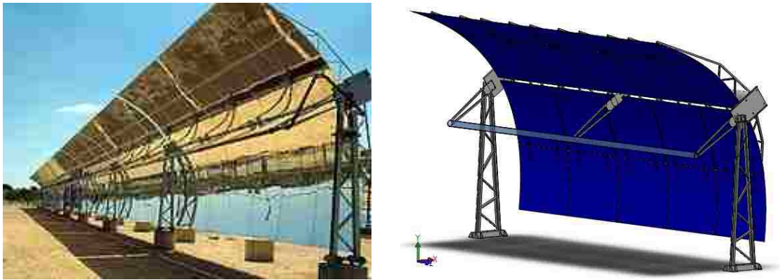
Figure 7. (Top) Photograph of actual LS-2 trough [3]; (Bottom) SolidWorks® model of LS-2 trough.
