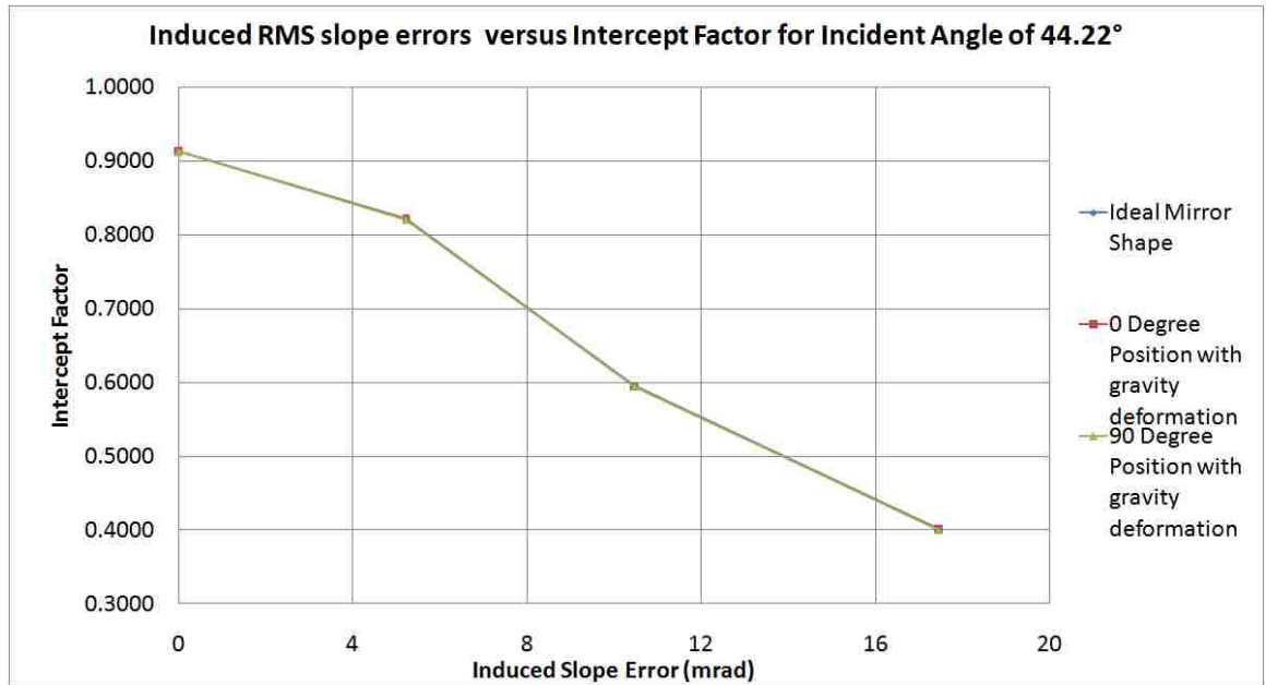
Figure 24. Intercept factors with increasing additional slope errors present on the reflective surfaces for the incident angle of 44.22° for the deformed models and ideal model
