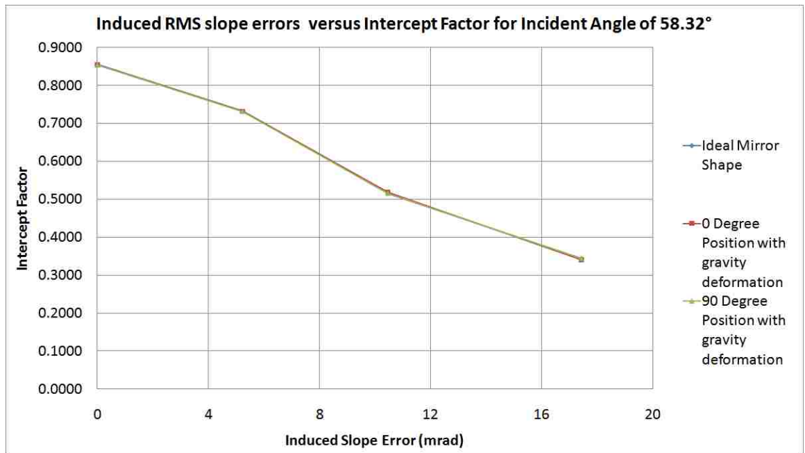
Figure 25. Intercept factors with increasing additional slope errors present on the reflective surfaces for the incident angle of 58.32° for the deformed models and ideal model
