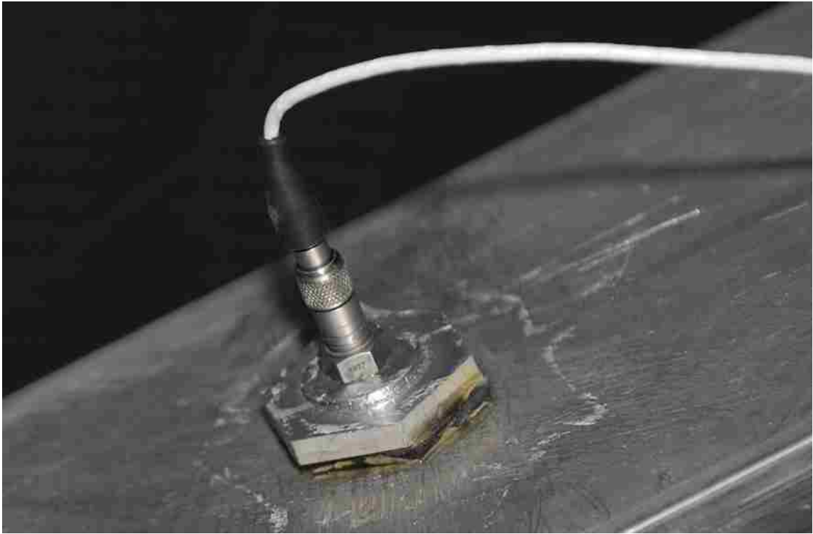
Figure 4.16: Pressure transducer mounted to driver section in isolation adapter
