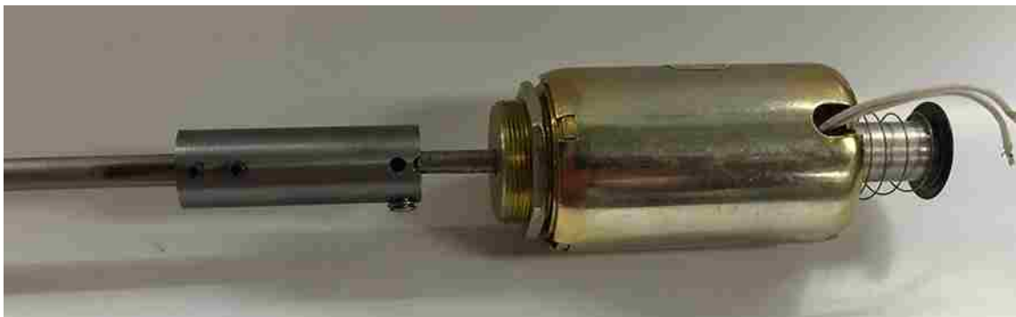
Figure 4.7: Close up of new coupler and solenoid, partially extended
