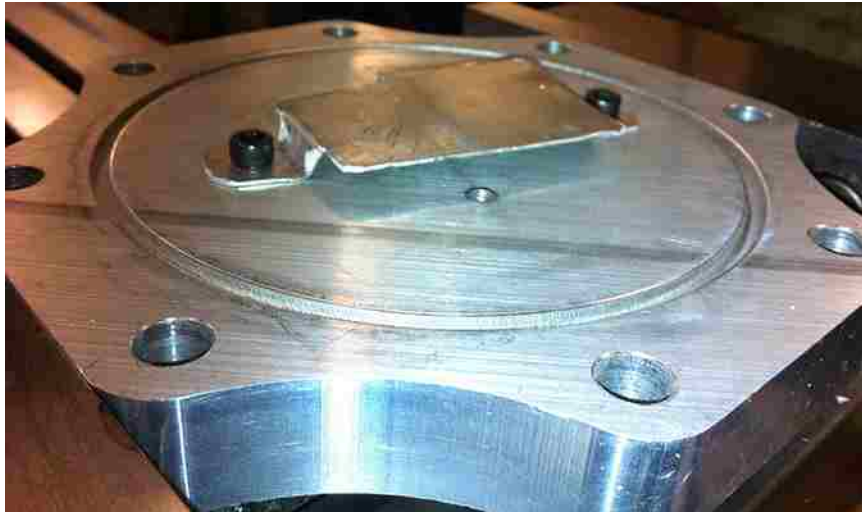
Figure 4.10: Baffle installed on flange
