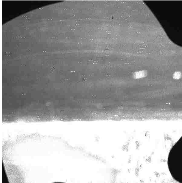
Figure 1.8: Particle Image Velocimetry with the iris just opening and three laser pulses
