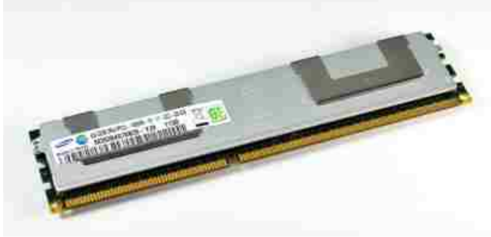
Figure 4: Samsung's 32 gigabyte DDR3 memory module with 3D TSV packaging technology [9].
