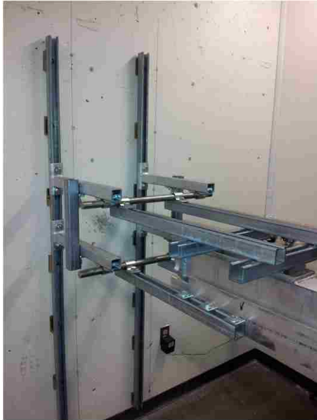
FIG. 15. Wall mount system setup for planar shock waves.
