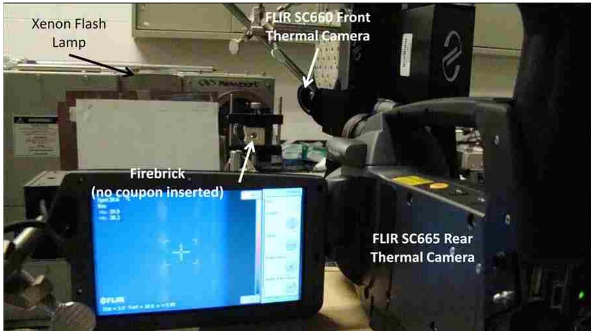
**Figure 3-6: Rear View of Experimental Setup Showing the Thermal Camera in the Back Orthogonal to Firebrick and Coupon**
