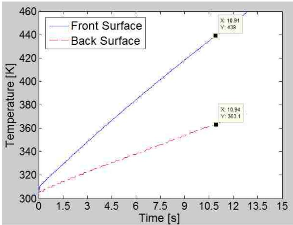
**Figure 4-7: Temperature Profile of Epoxy Polyamide Primer Surface and 2024-T4 Aluminum Substrate Surface. Incident Power  $18 \frac{W}{cm^2}$ , time to degradation 10.9s and 12.8s total exposure.**
