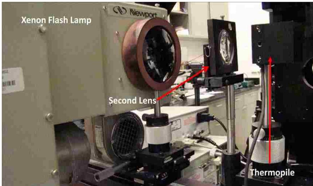
Figure 3-4: Energy Measurement Configuration
