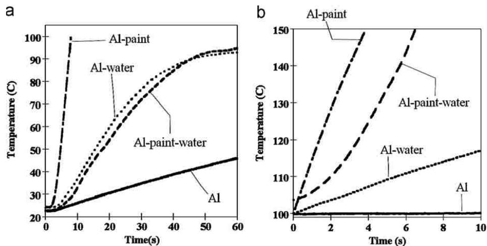
**Figure 2-4: Aluminum Back Surface Response to CO<sub>2</sub> 0.39kW/cm<sup>2</sup> Laser Courtesy of Y.H. Kim et al.**
