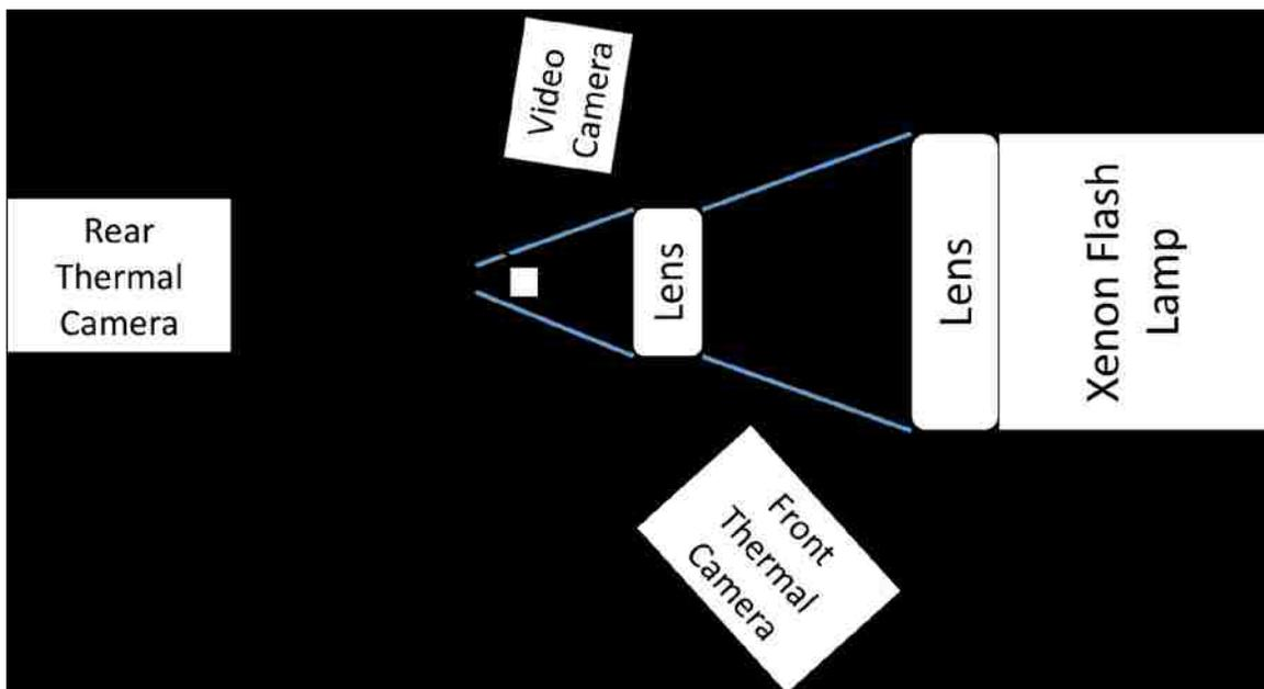
**Figure 3-8: Schematic Top View of Cameras, Coupon, Beam and Xenon Flash Lamp Locations**
