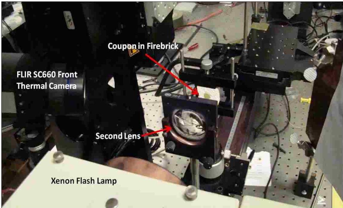
**Figure 3-9 Setup of Experiment in Nearly Ready Configuration.**
