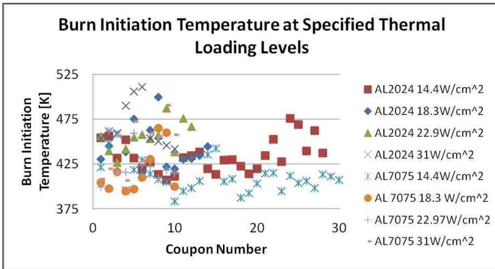
Figure 5-2: Mean Temperature of Burn Initiation Grouped by Incident Thermal Flux and Aluminum Substrate Type
