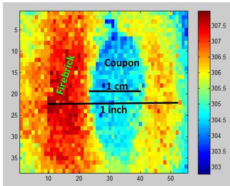
**Figure 3-5: The thermal camera in the front Image of Laser Initiation showing Laser is 1 Inch in Diameter and Firebrick is not Conducting Heat to or from Coupon**
