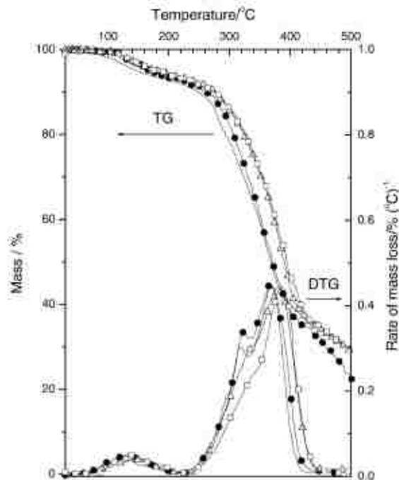
**Figure 2-3: Temperature Profile of Epoxy Maleate of Bisphenol A degradation, provided by Rosu et al.**
