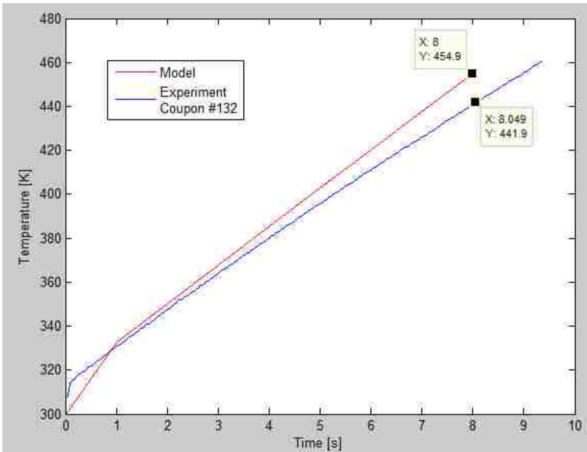
**Figure 5-5 Comparison of the Model and Experimental Measured Temperature Data from the 132<sup>nd</sup> Coupon Exposed with a 2024-T4 substrate and a 18W/cm<sup>2</sup> Exposure for 8 seconds**
