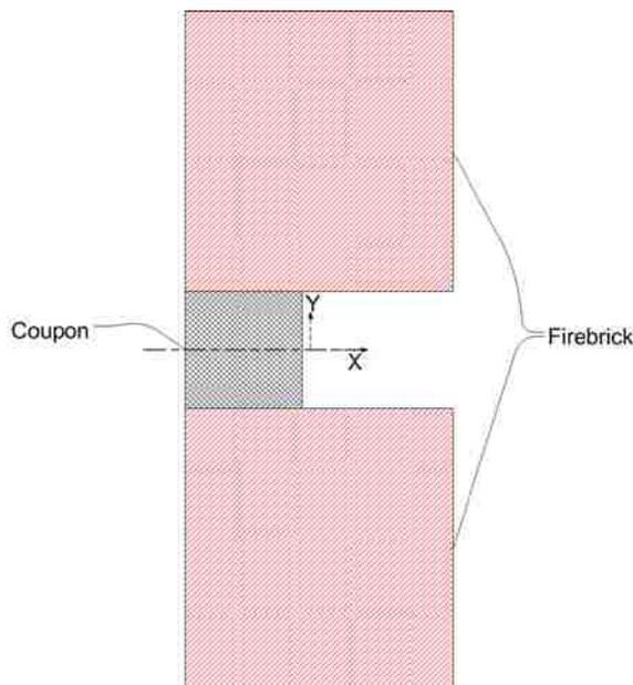
**Figure 1-1: Schematic of the Coupon Inside the Insulating Firebrick**
