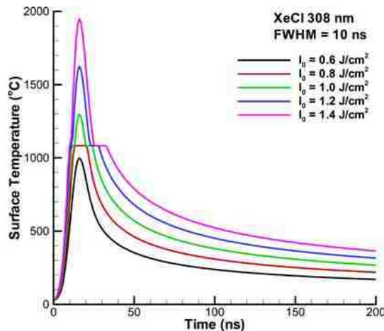
Figure 2-1: Temperature Profile of the Copper Substrate
