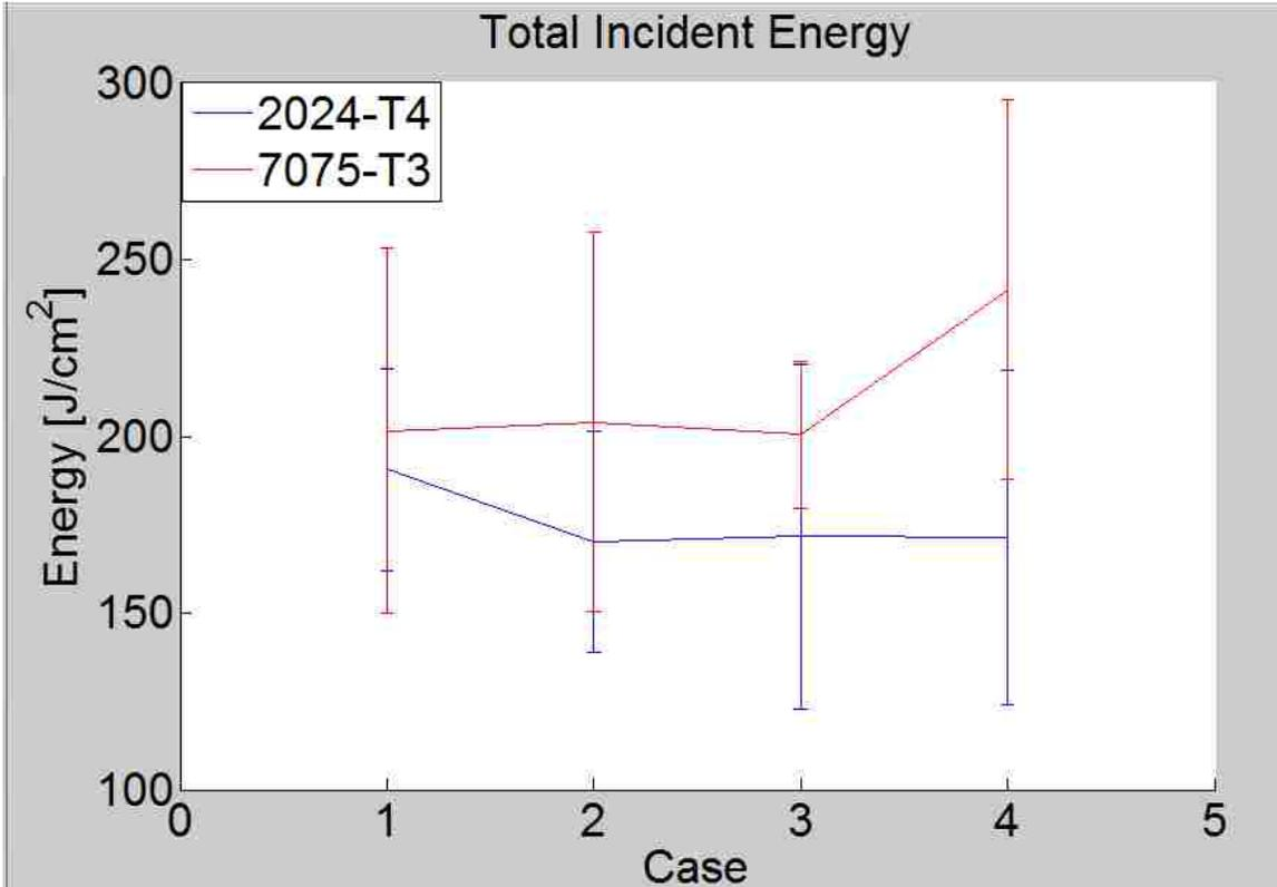
**Figure 5-4: Incident Energy for Initiation of Epoxy-Polyamide Primer Degradation on 2024-T4-T4 Aluminum Substrate with Margin of Error Bounds Included**
