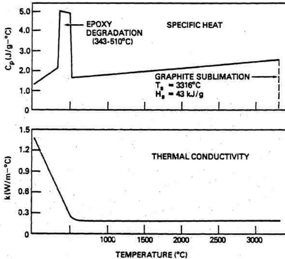
Figure 2-2: Epoxy Properties at different temperatures provided by the Naval Research Laboratory Griffis et al.
