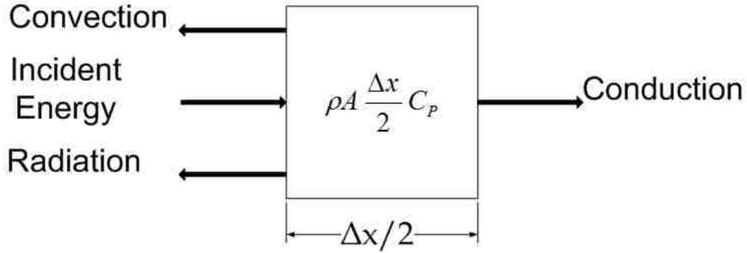
**Figure 1-3: First Node for FTSC Model with Boundary Conditions**
