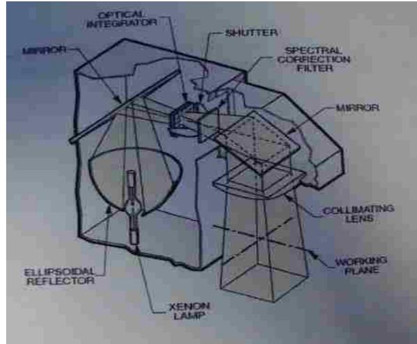
Figure 3-3: Schematic of how Xenon Flash Lamp Light is Emitted.
