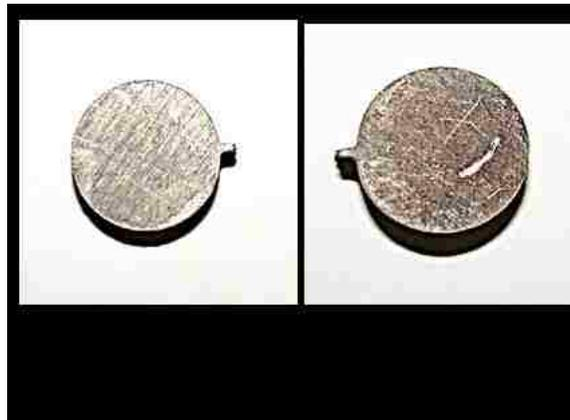
**Figure 5-6: Surfaces of 2024-T4 and 7075-T3 Aluminum Substrates**
