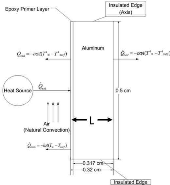
where the back surface shows negligible convection that is discussed in the results section. The aluminum was not exposed to free flowing air on the non-coated backside, but there is still convection. The true amount of convection at the back surface is not easily calculated and is assumed to
