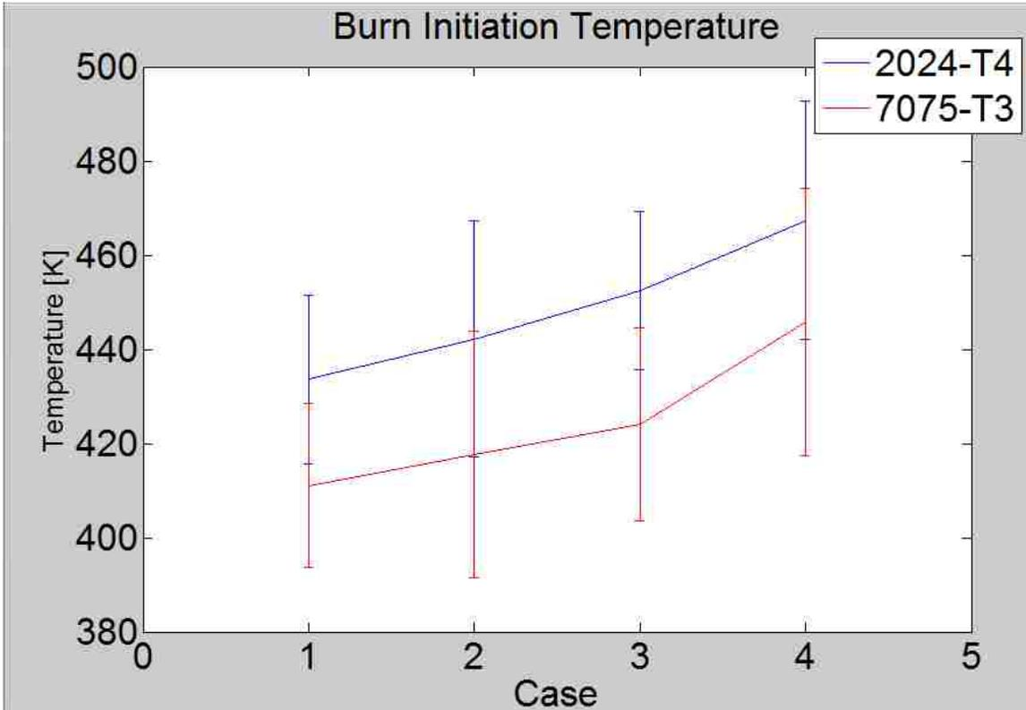
**Figure 5-3: Burn Initiation temperatures Plotted with Error Bounds for Epoxy Polyamide Primer coated Aluminum 7075-T3**
