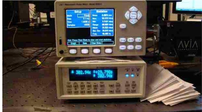
**Figure 3-7: Newport Thermopile Control Box, Display Energy in  $W/cm^2$  for different bulb power settings**
