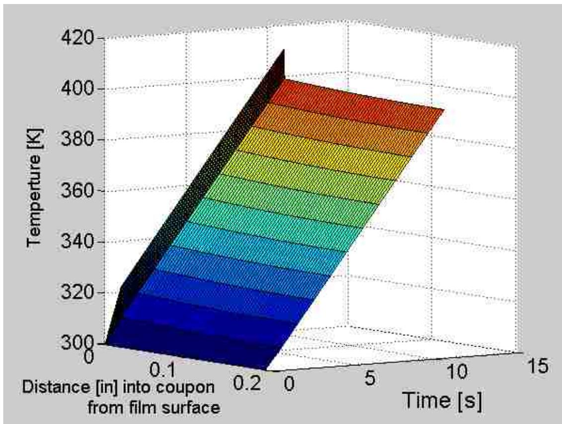
**Figure 5-7: Modeled Coupon Volume Based on Temperature at Nodes for Degradation for a 18 W/cm<sup>2</sup> Incident Flux for 11 seconds of an Epoxy Polyamide Coated 7075 Aluminum Substrate**
