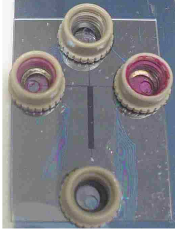
Figure 36: Photograph of a standard T-Chip type device that is used in experimental efforts. Note the nanoport reservoirs are bonded to the surface of the chip to allow for sample injection. Since this is a used chip, the left and right wells are discolored from the proteins/dyes that have collected in the respective reservoirs.
