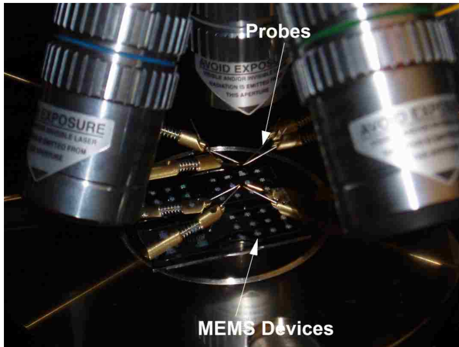
Figure 18: Probe tips in contact with bonding pads of a MEMS actuator
