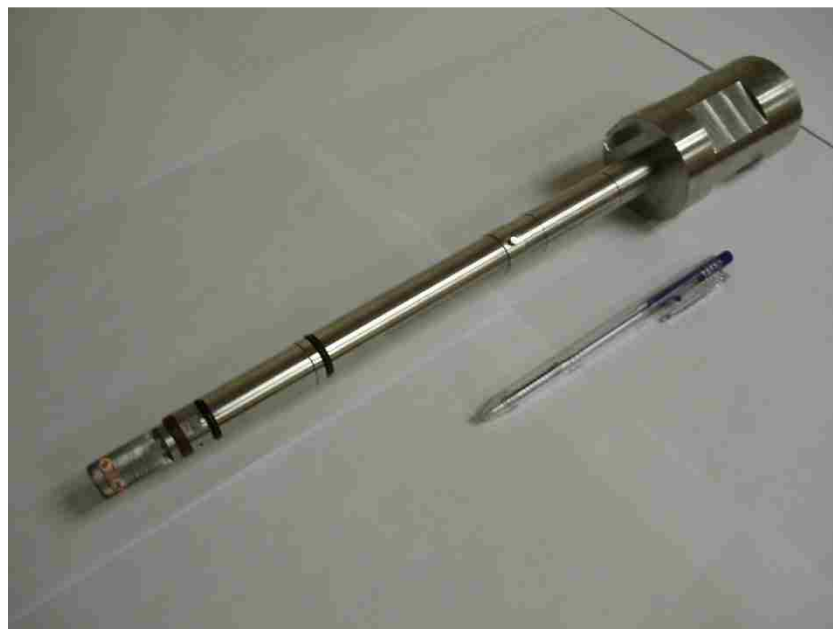
Figure 12: Custom manufactured TEM holder
