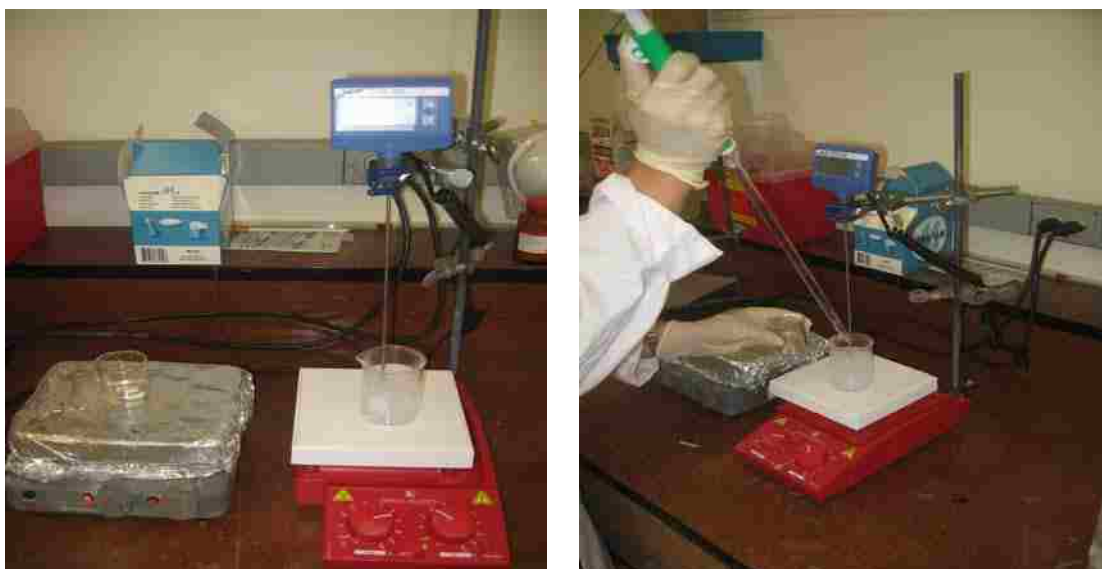
Fig 2.2 Dissolve solutions (left) and mix them (right) during the synthesis of LaF 3 : Ce Nanocrystals
