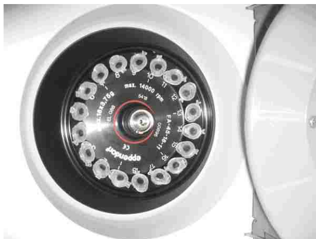
Fig 2.4 Use of centrifuge to separate \text{LaF}_3 : Ce nanocrystals from colloidal solution 0%, 1% and 10% \text{Ce}^{3+} -doped \text{LaF}_3 nanocrystals were prepared by using this method as well; stoichiometrically.
