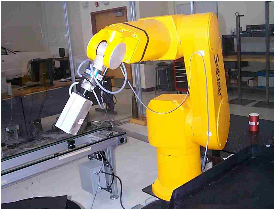
Figure 3.5. Staubli RX-130 robot carrying a laser pointer tool.
