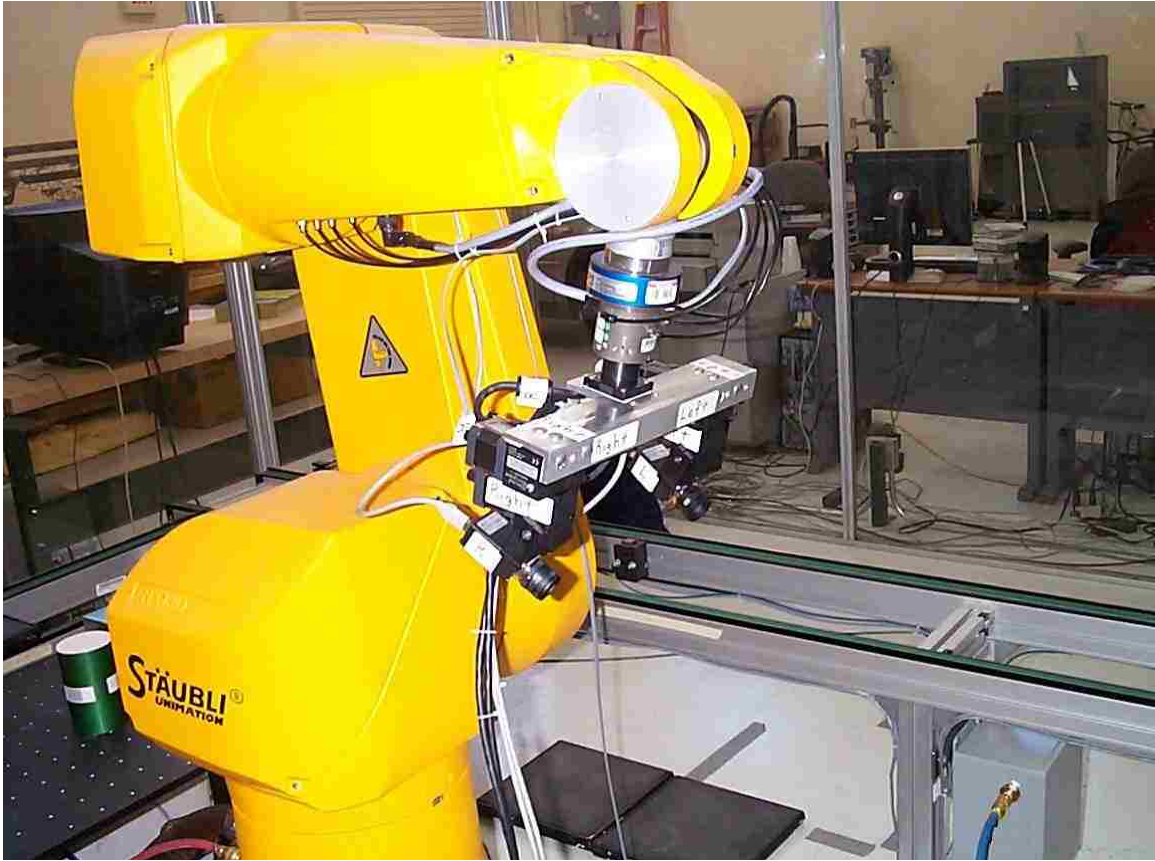
Figure 3.8. Staubli RX-130 robot carrying Biclops.
