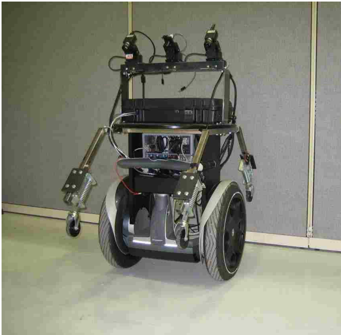
Figure 3.14. Segway Robotic Mobile Platform with Biclops Directed Vision System.
