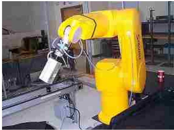
Figure 6.1. Staubli RX-130 robot carrying a laser pointer tool.
