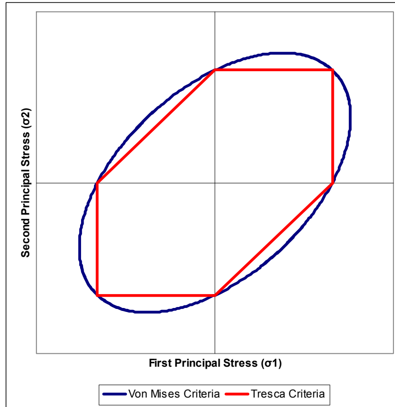
Figure 4-1: Tresca and von Mises Yield Criteria
