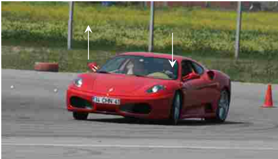
Figure 1.1 – Example of Lateral Load Transfer
