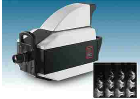
Figure 3.11: DRS Imacon 200 ultra-high speed camera, captures 14 frames from 1000 to 200 million frames-per-second [19].
