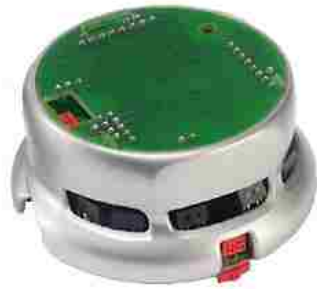
Figure 5.2: The Khepera II mobile Robot
