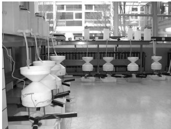
Figure 2 Photo of rain gauge calibration.
