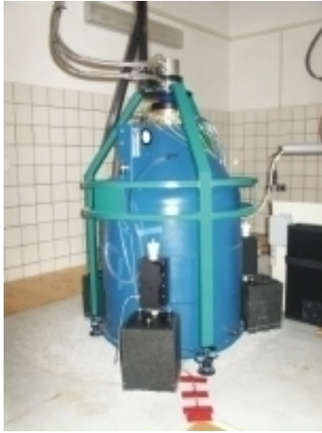
Figure 1.2: The superconducting gravimeter at the Geodynamic Observatory Moxa, Germany.
