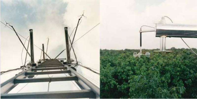
Figure 4.1: The picture at the left shows the ladder mounted on top of the scaffolding tower and 3 of the 4 trolleys with dry and wet bulb temperature sensors. The cup anemometers are at a fixed height. The picture on the right shows a cup anemometer and the inlet for the aspirated temperature sensors.
