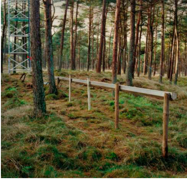
Figure 4.4: The 10 m long and 10 cm wide throughfall gutter at the Loobos site, with at the end (just behind the left tree) the tipping bucket gauge.
