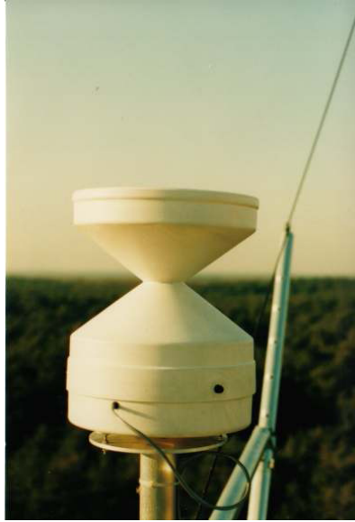
Figure 4.3: The champagne glass shaped tipping bucket rain gauge as has been used at all sites, except Edesebos site, on top of the tower and in the open field.
