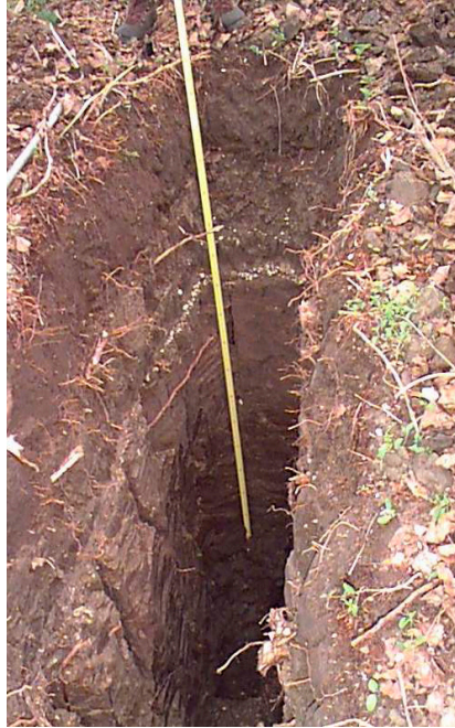
Figure 3.14: The soil profile at the Fleditebos site showing 3 distinctive layers. On top of the deepest layer sea shells are present. The large cracks that occurred after the land was reclaimed from the sea, can clearly be seen at the left side of the pit. The length of the tape in the photograph is 1.7 m.
