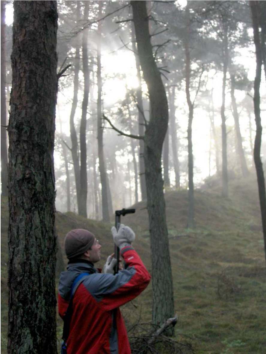
Figure 3.2: Employment of the LAI-2000 sensor below the canopy to measure the leaf area.
