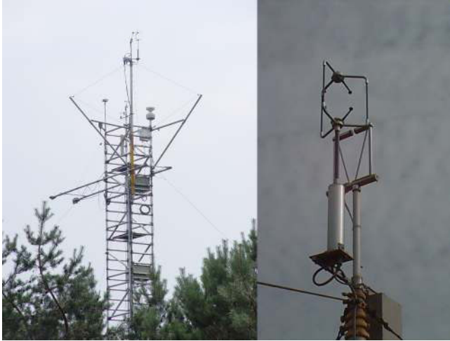
Figure 4.2: The left picture shows the top of the scaffolding tower, with the eddy-correlation system at the top of the extendible mast, rain gauge, temperature/humidity sensor, cup anemometer and wind direction sensor on top of the scaffolding tower and the radiation sensors extending 3 m horizontally out of the tower. The right picture shows the 3D-sonic anemometer and the krypton hygrometer of the eddy-correlation system.
