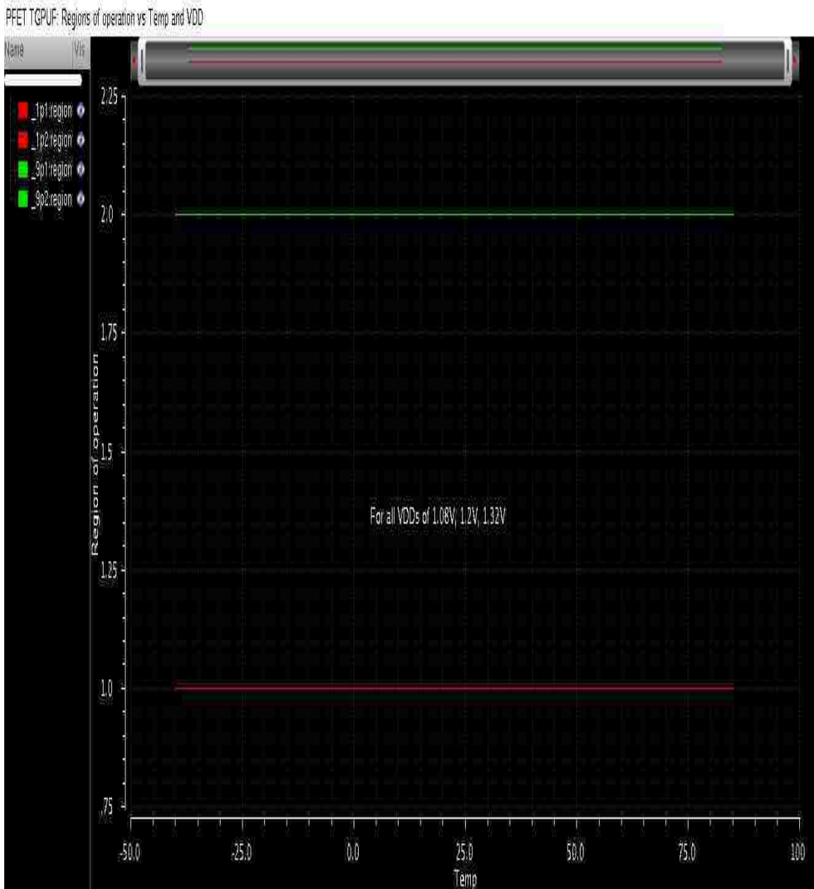
Fig. 117. PFETs 1p and 9p regions of operation at the 9 TV corners
