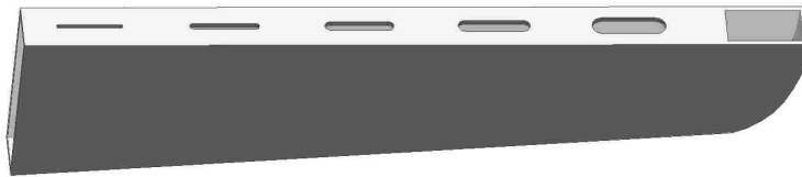
Figure 6.1: Modified narrow-wall longitudinal-slot array for higher gain.
