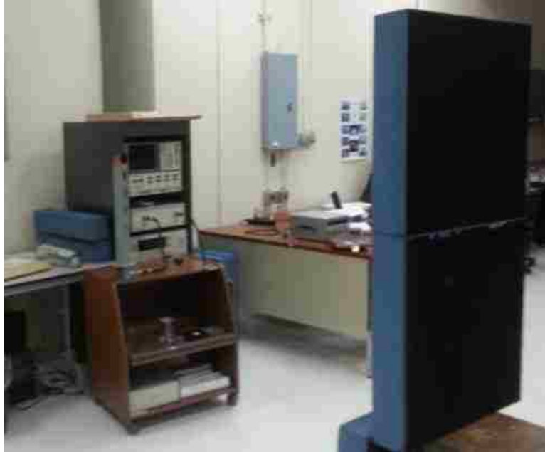
Figure 5.2: Experimental set-up for measuring reflection coefficient using the network analyzer.
