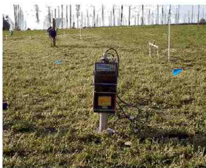
Figure 2.4. Neutron scattering probe (Muñoz-Carpena et al., 2006)
