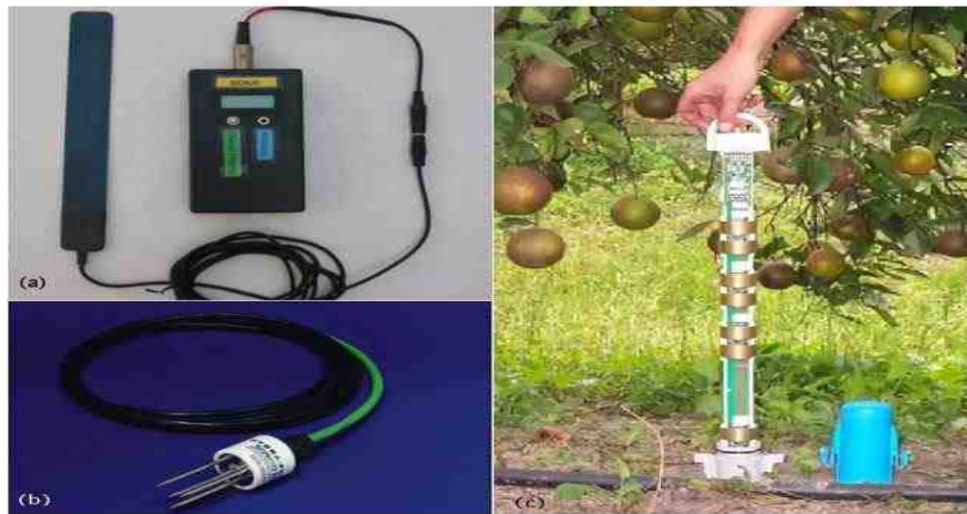
Figure 2.6. FD probes (a) Capacitance (plates) (b) Capacitance (rods) and (c) FDR (rings) (Muñoz-Carpena, 2002)
