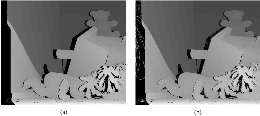
Figure 5.9: Illustrating step# 4. (a) shows the disparity map with the occluded areas (b) shows filled occluded area with the edge map depending on the type of occluded areas.
