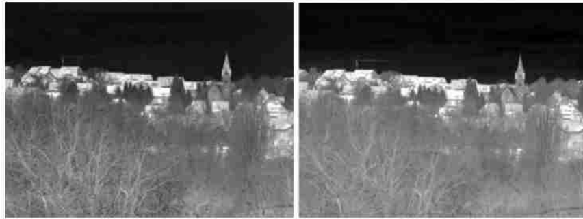
Figure 1.5: Images taken with a dual band QWIP FPA [2]. The left image shows the scene in the MW and the right image shows the same scene in the LW.
