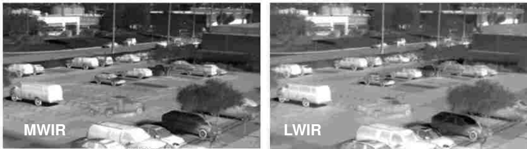
Figure 1.2: MWIR and LWIR images taken with two-color HgCdTe FPA [2]
